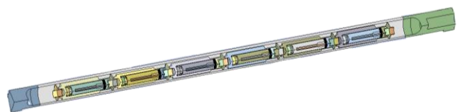
Fig. 3. Quarter-symmetry ANSYS target model.
