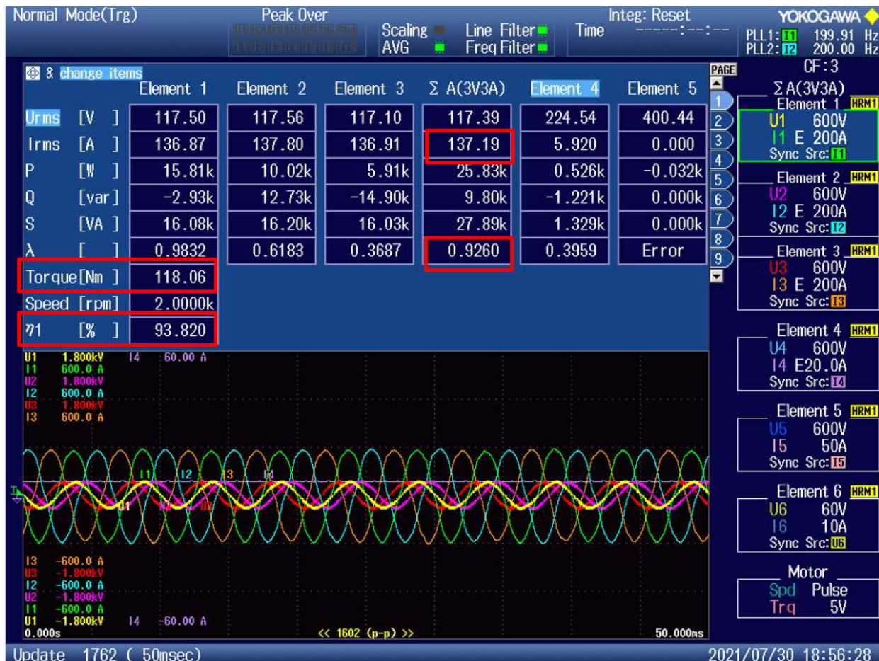
Fig. 2.6.3-1. Yokogawa WT1800 power analyzer screen capture of operation near load point 3 conditions. The first three elements are the stator phases. The sigma element is the aggregated behavior of the three elements and the fourth element is the field excitation. The fifth element is the DC link voltage from the power interface unit.
