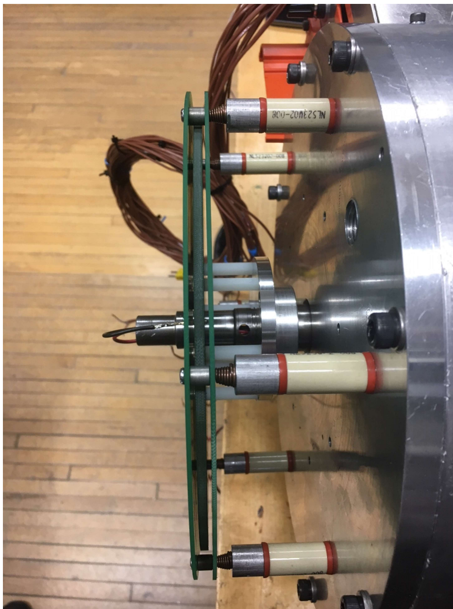
Fig. 2.4.4-8. Three phase Rev 1 PCB CPC mounted on WFSM non-drive end bell with insulating standoffs and press-fit rotor hub.
