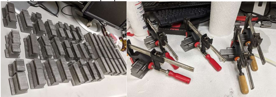
Fig. 2.3.7-6. Damaging poles from shipment and repair thereof.
