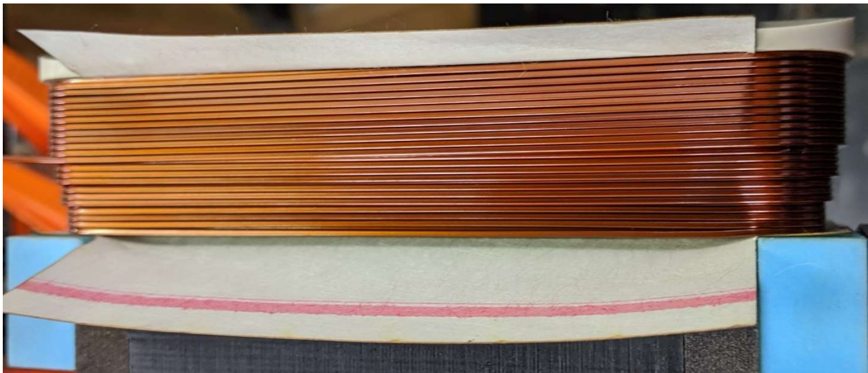
Fig. 2.3.7-9. Winding of square 19 AWG equivalent magnet wire onto pole stack.
