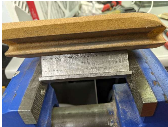
Fig. 2.3.7-7. Dovetail grinding using precision 3D printed hand grinding block.
