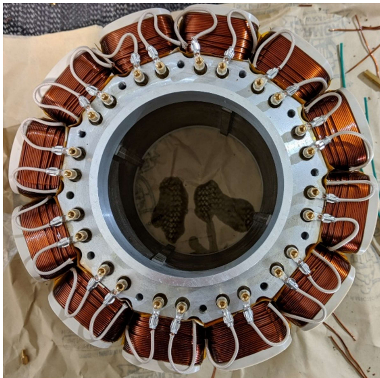
Fig. 2.3.7-15. View of complete rotor after vacuum pressure impregnation without the shaft.
