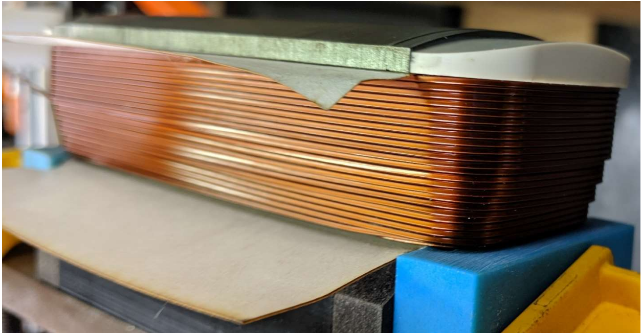
Fig. 2.3.7-10. Alternative view of winding of square 19 AWG equivalent magnet wire onto pole stack.
