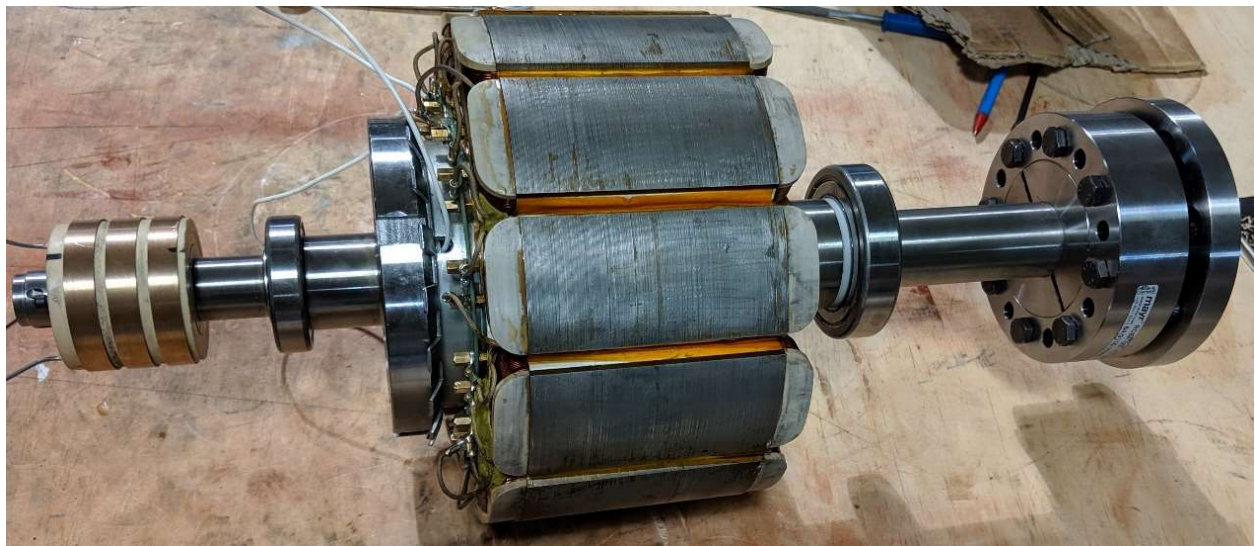
Fig. 2.3.7-17. Complete rotor assembly after balancing.
