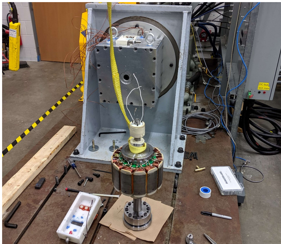
Fig. 2.6.2-2: Preparing to insert the rotor assembly into the housing.
