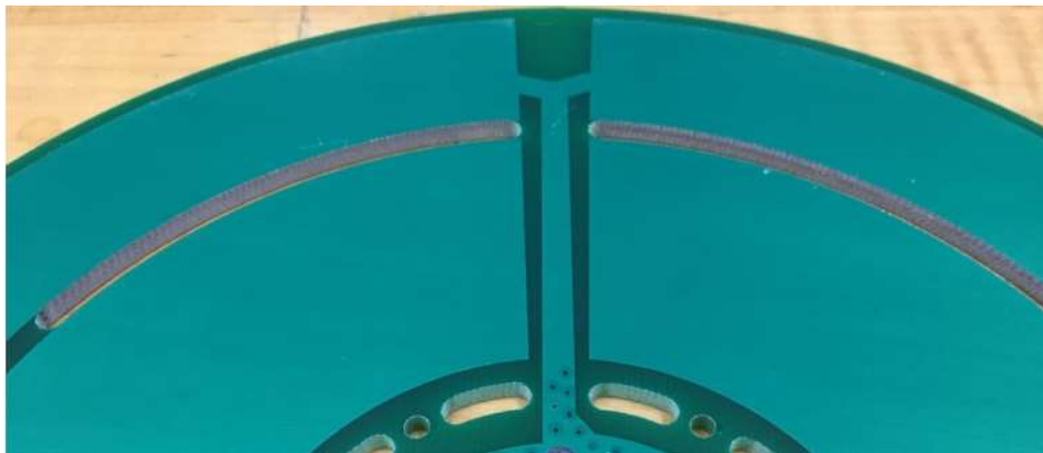
Fig. 2.4.4-13. Example 2-layer rotor CPC with connection from outer electrode through gap in inner electrode to rectifier near inner radius.
