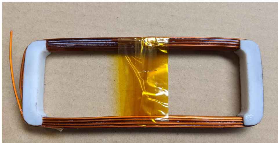
Fig. 2.3.7-21. Trial twisted square wire coil with modified endcaps.
