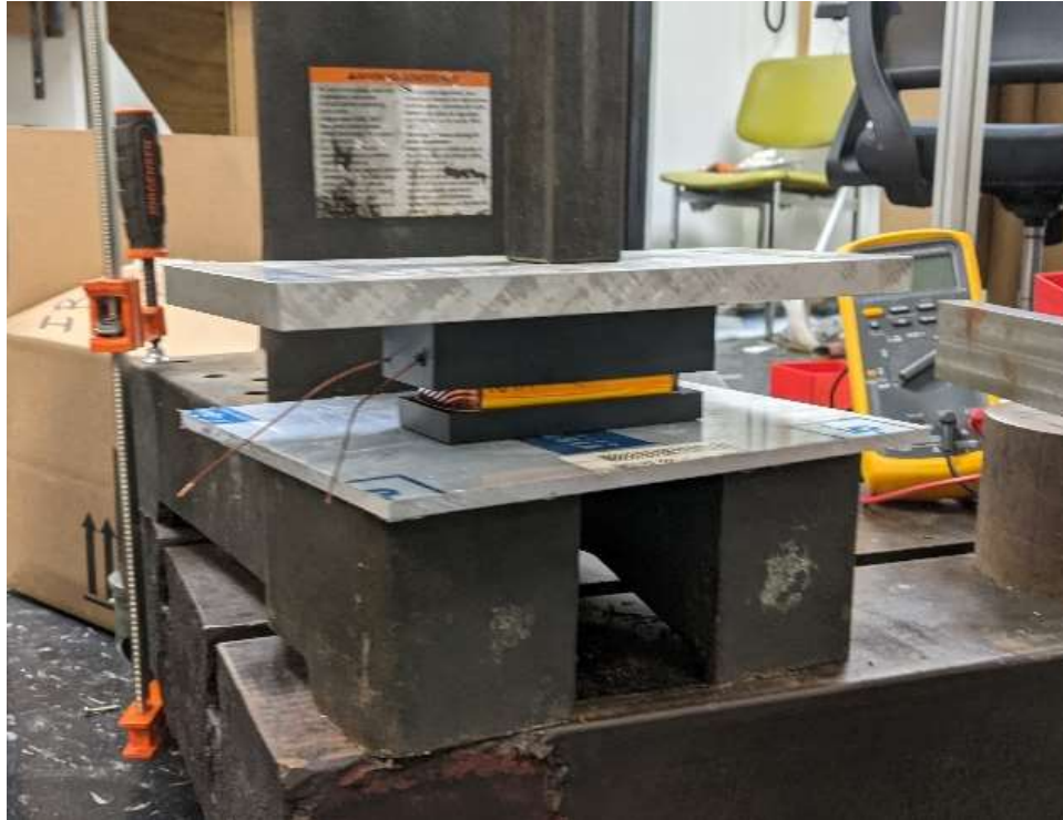
Fig. 2.3.7-12. Winding consolidation on salient pole.
