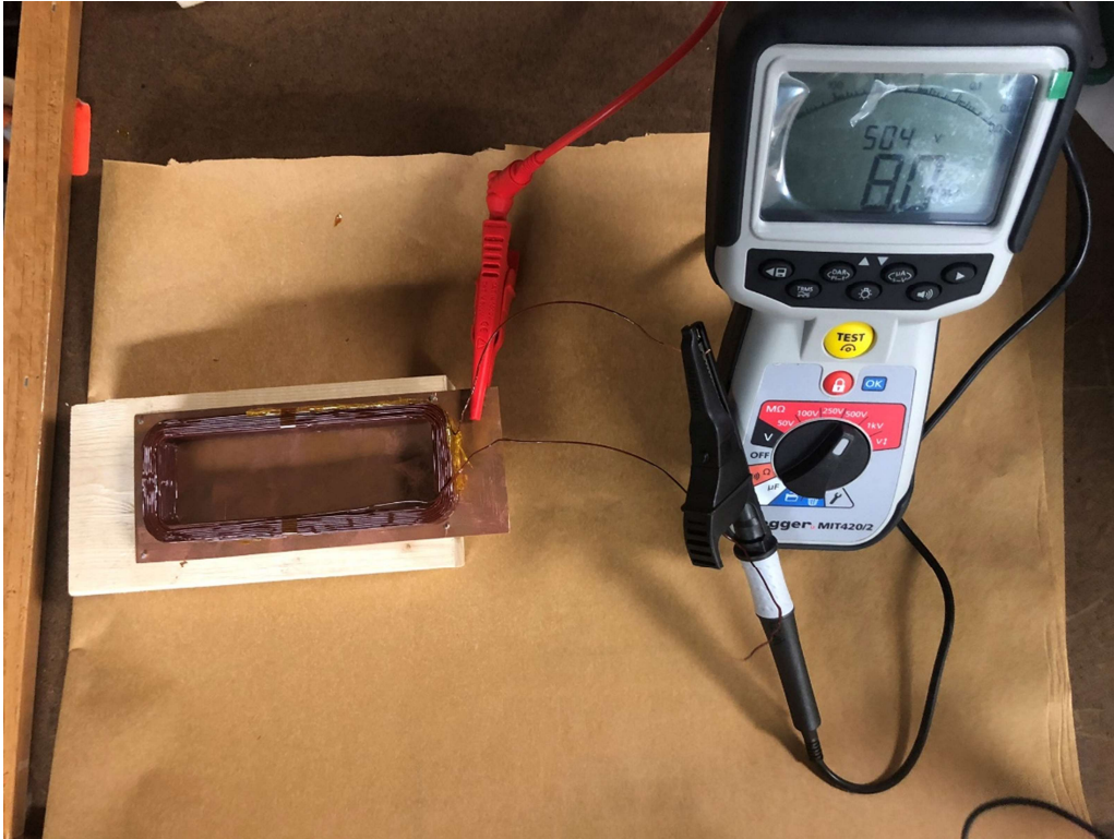
Fig. 2.2.3-10. HIPOT and surface insulation tests of die compressed coils.
