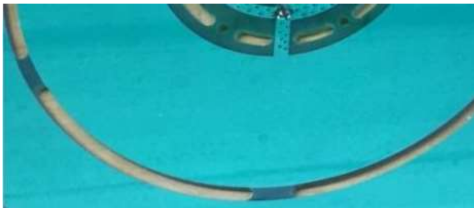
Fig. 2.4.4-11. Example slotting between adjacent CPC electrodes to reduce dielectric losses.
