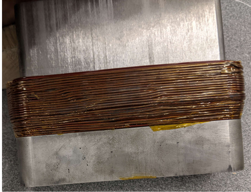
Fig. 2.3.7-32. Compressed coil on bobbin after compression.
