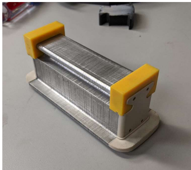
Fig. 2.3.7-8. Alignment and epoxying of PEEK endcaps onto pole piece lamination stacks.
