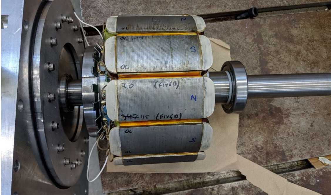
Fig. 2.6.2-3. Installation of the rotor assembly into the housing. The non-drive end plate is visible.
