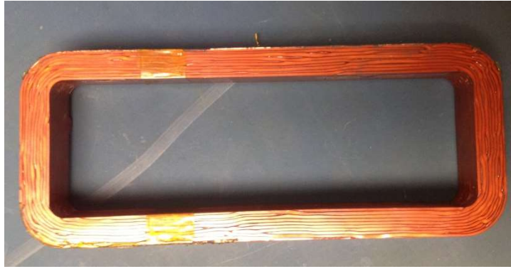
Fig. 2.2.3-6. Representative die compressed coil for generation II WFSM
