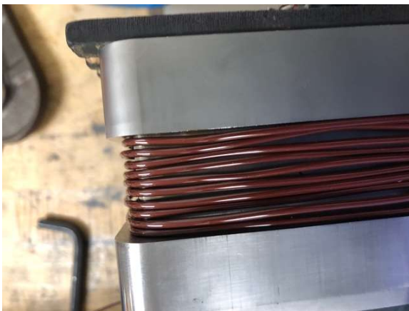
Fig. 2.3.4-4. Initial trial coil with two strands per turn of 11 AWG magnet wire.
