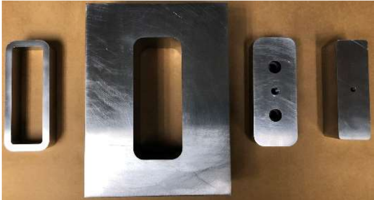
Fig. 2.2.3-3. Die used to produce compressed field coils for generation II WFSM.
