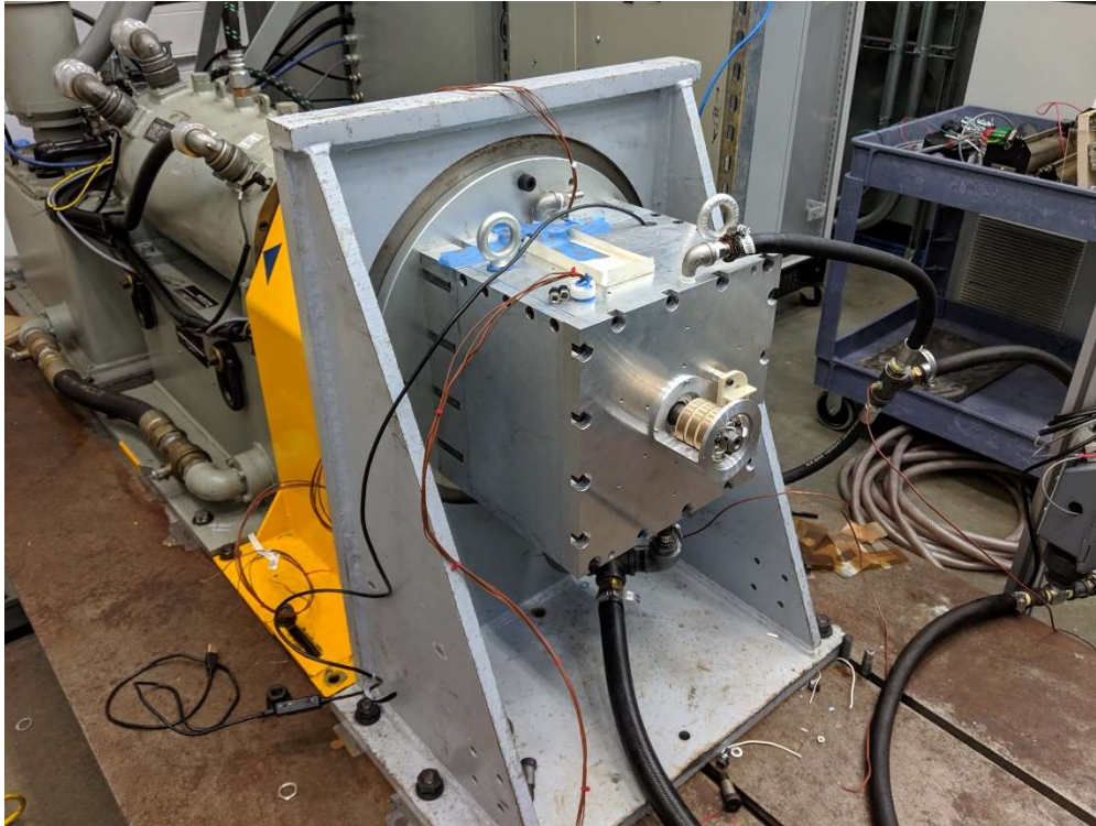
Fig. 2.6.2-5. WFSM prototype mounted and aligned with partial cooling system connections and encoder mount installed.
