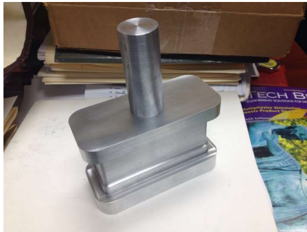
Fig. 2.2.3-2. Aluminum bobbin for trial winding of coil before compression.
