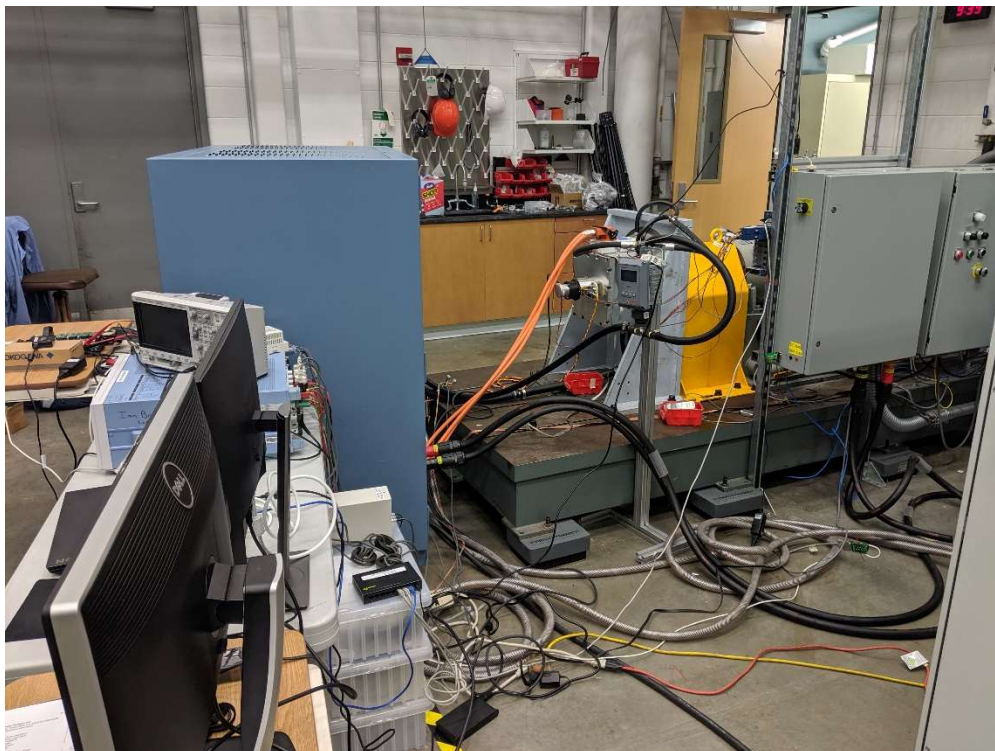
Fig. 2.6.2-19. Final testing setup with brushes and slip rings
