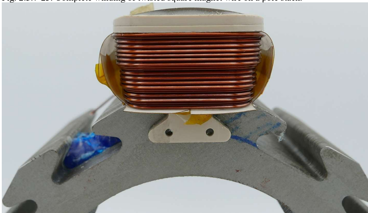
Fig. 2.3.7-26. Salient pole with twisted square wire inserted into pole stack.
