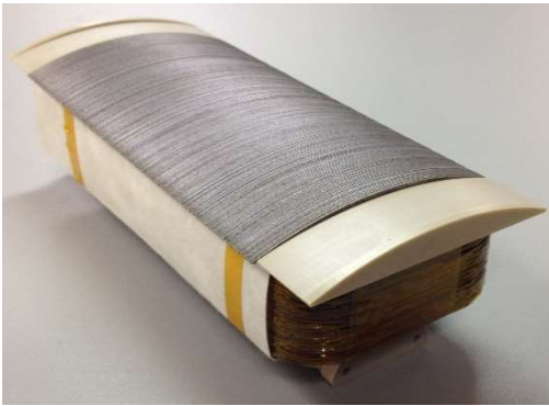
Fig. 2.2.3-7 Segmented rotor pole and pole mounted on rotor yoke.
