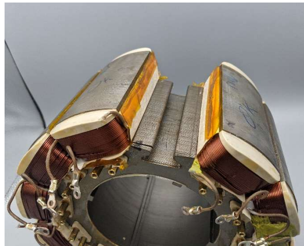
Fig. 2.6.4-9. Evidence of arc flash damage to rotor pole and laminations after extraction of damaged rotor pole.
