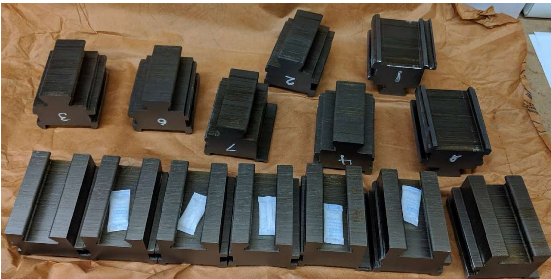
Fig. 2.3.4-9. Cut apart positive and negative dovetail pieces.
