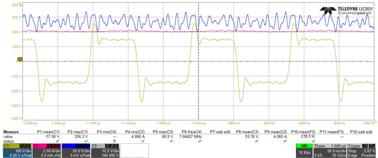
Fig. 2.6.4-6. Operation of the CPC powering the WFSM field at a switching frequency of \sim 7.1 MHz and 4 A field current with the generation II high frequency single phase inverter. The yellow trace is the inverter output voltage and the pink trace is the field current.
