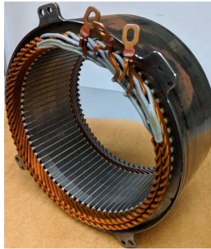
Fig. 2.3.6-1. GM Chevy Volt Gen 1 motor B stator.
