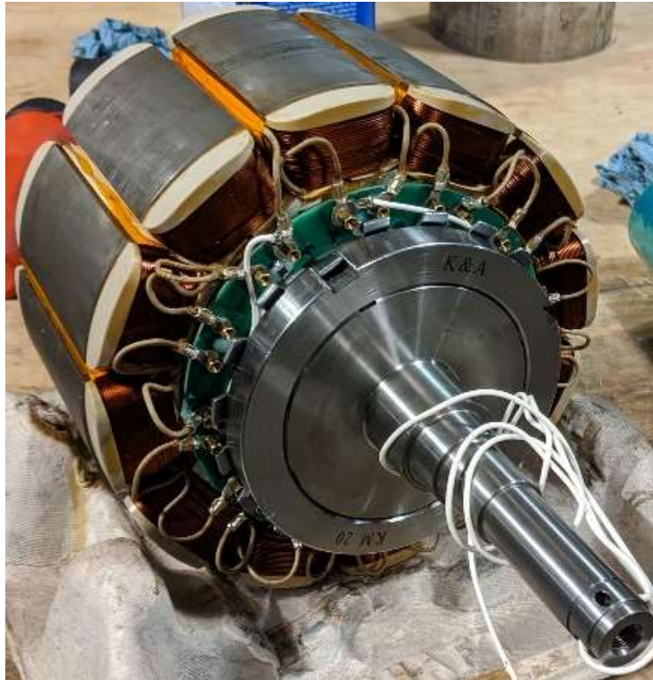
Fig. 2.3.7-16. Rotor mounted on shaft with connection PCB.
