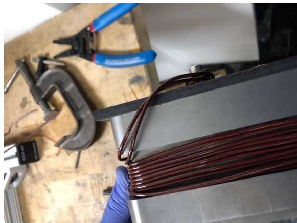
Fig. 2.3.4-4. Initial trial coil with two strands per turn of 11 AWG magnet wire.
