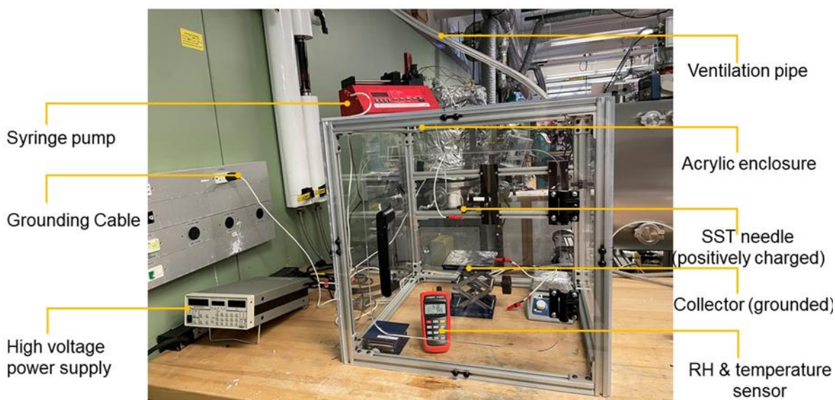
Figure 36. Customized electrospinning setup for fabricating hydrophobic membranes.
