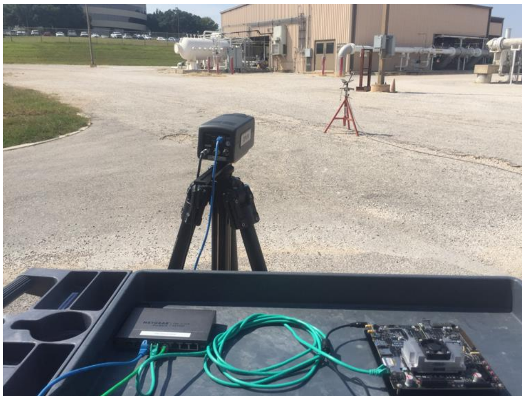
Figure 11. Image of setup used for data collection at various ranges, ambient conditions, and leak types
