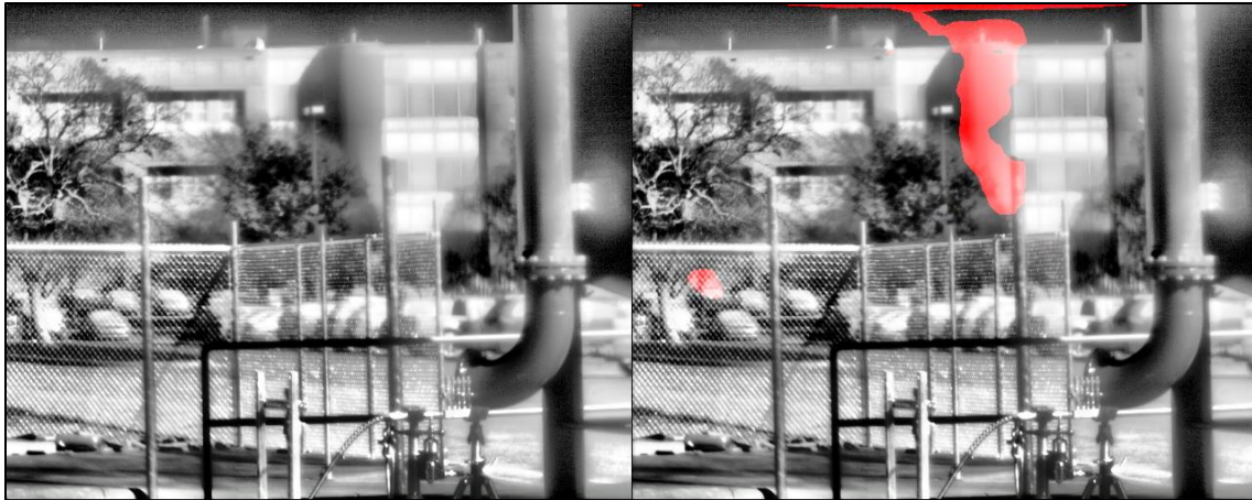
Figure 7. Comparison Showing Steady Tracking on Noisy Background, Methane Plume Not Apparent to Human Eye in Video
