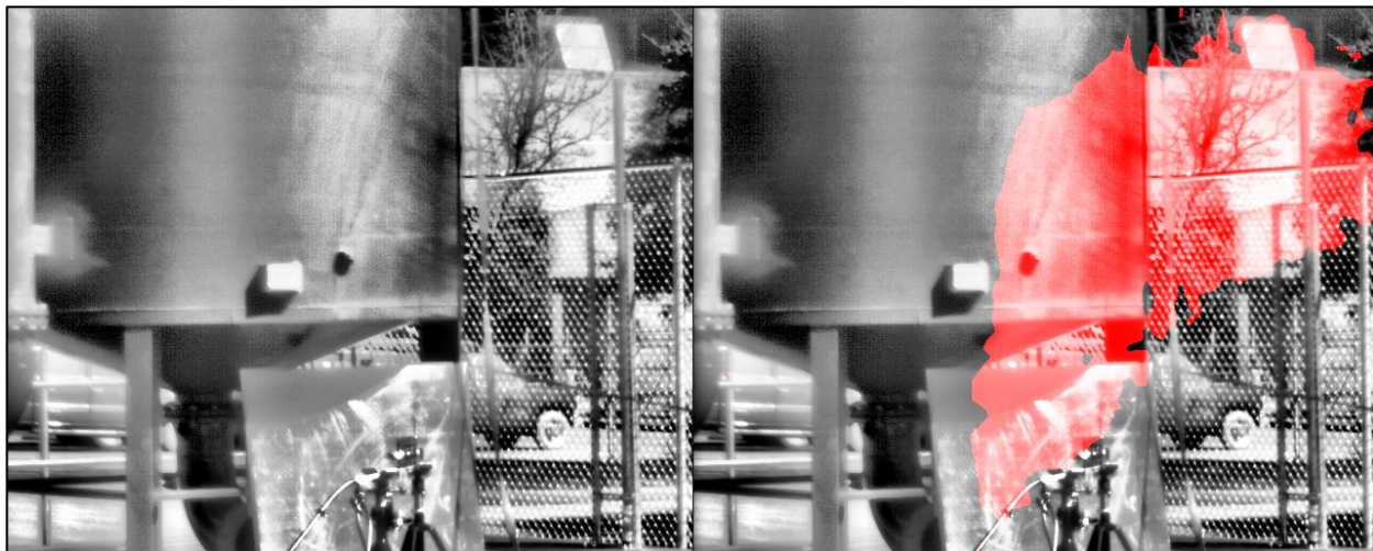
Figure 10. Comparison Showing Good Tracking on Solid Background Again, Failures Present on Bottom-Left of Highlighted Area: Problems Persist Where High-Reflectivity Background Converges with the Plume
