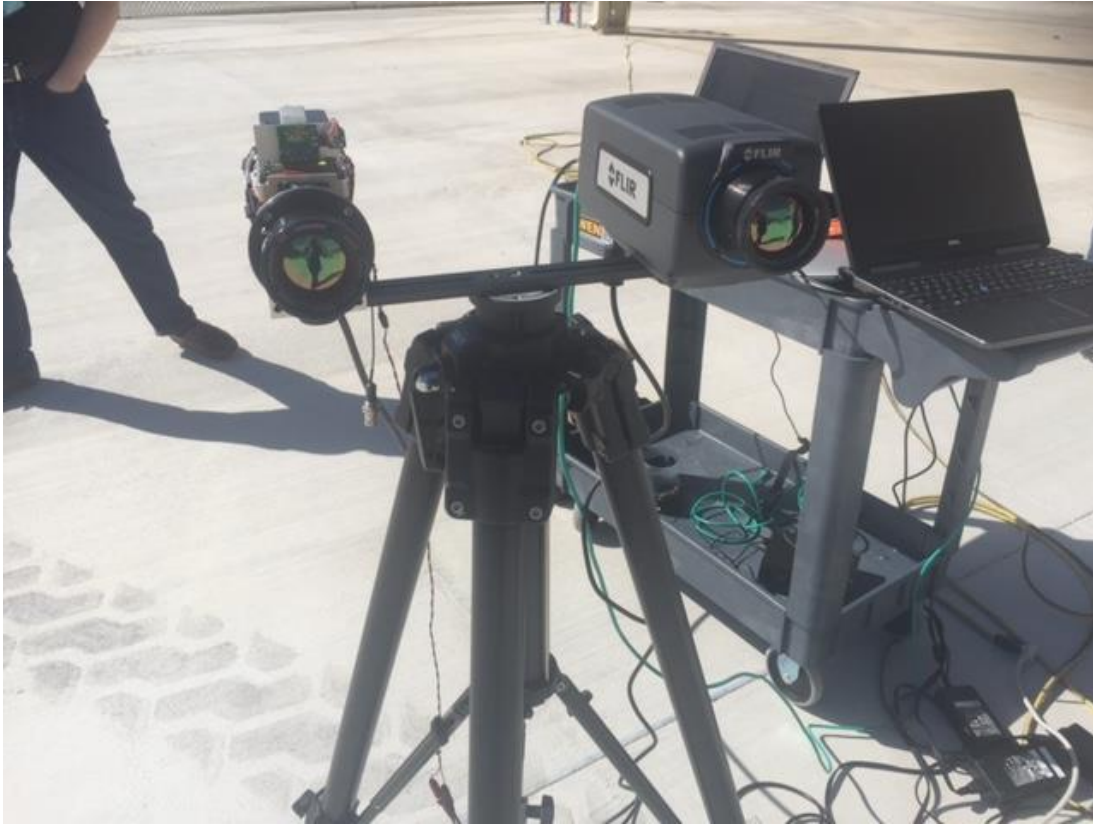
Figure 3. Niatros™ and FLIR MWIR Cameras Acquiring Data During a Supervised Methane Release
