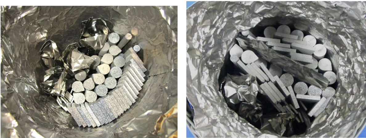
Figure 97. All samples from Builds 2 (left, paired with Build 1) and 6 (right, paired with Build 5) were Placed in the HIP Oven
