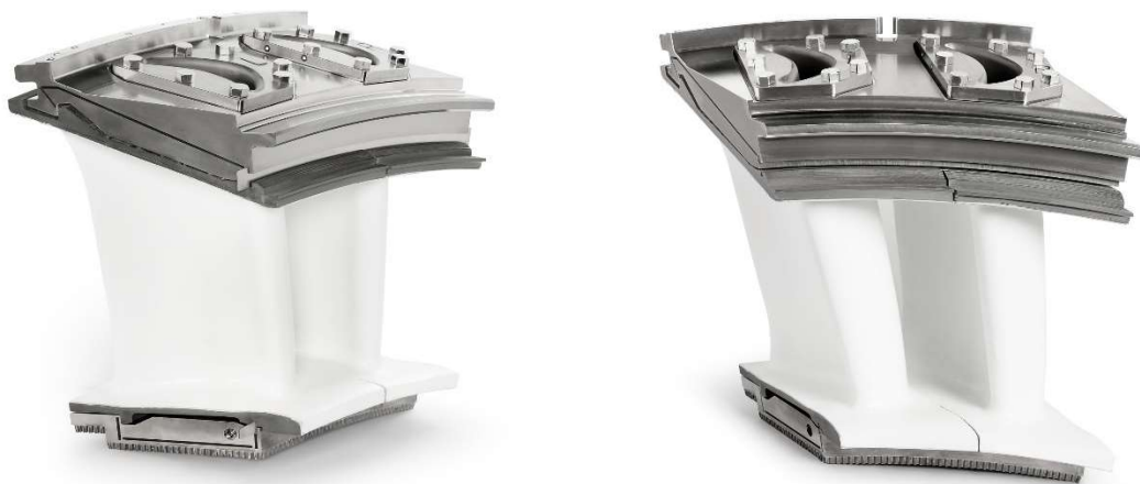
Figure 34 – Fabricated 2 nd stage CMC nozzle segment
