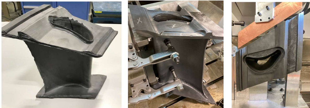
Figure 29 – Unmachined CMC fairing, grind setup, EDM setup
