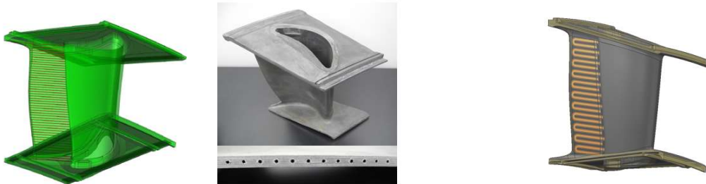
Figure 27 – Straight holes and stacked serpentine passages
