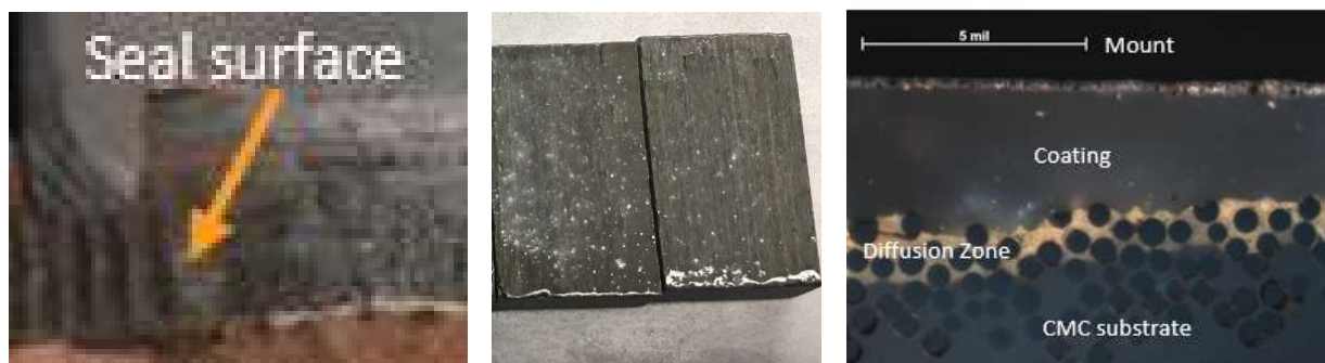
Figure 15 – CMC as machined seal surface, coated CMC and cross-section
