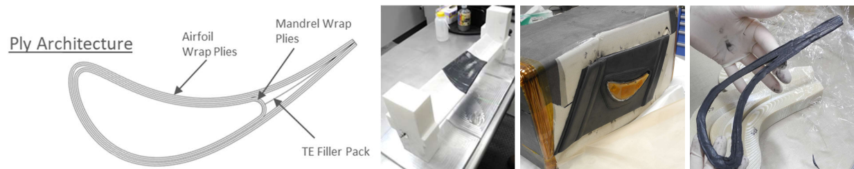
Figure 12 – CMC airfoil ply architecture with airfoil, end-wall, and tooling
