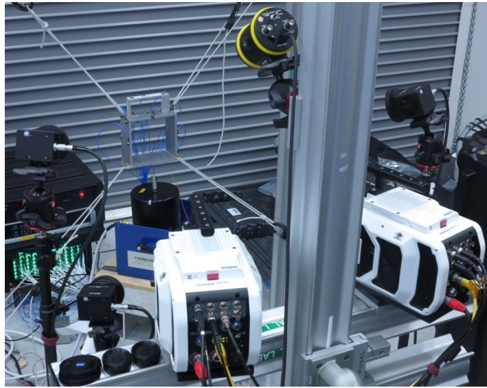
Figure 7: Example stereo DIC test of the BARC structure
