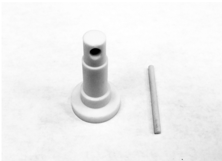
Figure 1. Alumina Specimen holder used for the SATS high-temperature steam oxidation tests.
