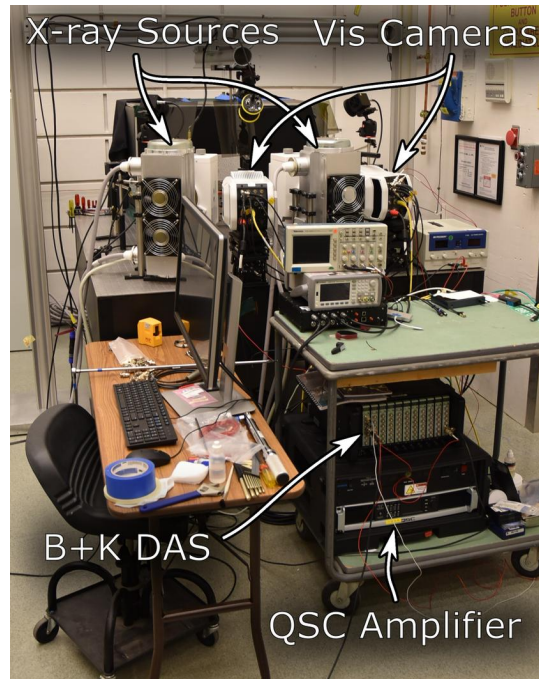
Figure 9: Test overview showing the data acquisition systems and shaker amplifier.
