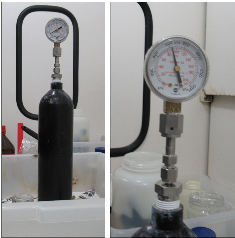
Figure 33. Reaction vessel for 1 L reaction of DMMP. After addition of the reagents, the temperature and pressure in the sealed steel container increased, shown by the pressure gauge on the right. The pressure eventually rose higher than 13.6 atm (200 psi), and the temperature of the outside was 171°C.
