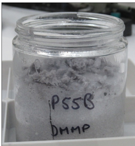
Figure 31. Final product for sample P55B. This order of addition caused rapid reaction, and the sample completely solidified in a few minutes.
