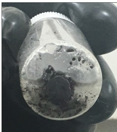
Figure 99. 4.0 mL of HD with pellet F09-138C and 0.4 mL H 2 O. The intact pellet can be seen at the bottom of the vial.
