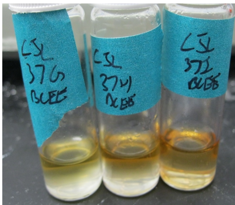
Figure 72: Reactions of BCEE with \text{Li}_3\text{N} and thiourea. The solution developed an orange coloration, but did not polymerize or exhibit other signs of surrogate decomposition.
