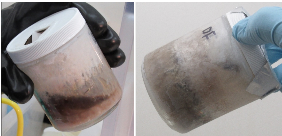
Figure 53. Reaction of 100 mL DF with water and \text{Li}_3\text{N} . Left:, after 10 days of reaction time (Sample nb0049P21A), right: after 2 months. The reaction product is initially a mixed liquid (brownish color) and solid (light brown). DF is not detectable by NMR after <1 day. The lid of the jar could not be removed, so a hole was cut in the lid to sample the product. After 2 months, the product is completely solidified.
