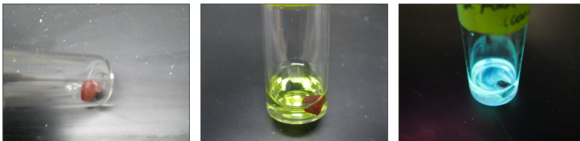
Figure 55. Images of wax-encapsulated fluorescein dye (left) in DPCP (center) under UV irradiation (right).
