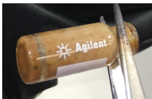
Figure 41. Reaction mixture of HD with \text{Li}_3\text{N} + \text{H}_2\text{O} (22% w/w), sample nb097P143D.
