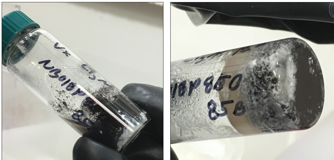
Figure 34. Reaction mixture of 10 mL VX + \text{Li}_3\text{N} + \text{H}_2\text{O} , using 10 mL VX, 9% \text{Li}_3\text{N} . Left: 3.5% \text{H}_2\text{O} after 5 days reaction time; Right: additional 5% \text{H}_2\text{O} after additional 5 hr and manual stirring.
