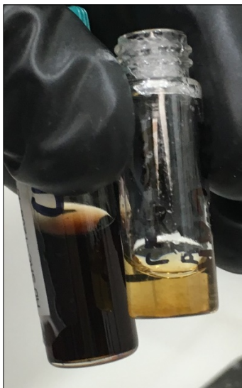
Figure 39. Reaction mixture of HD + \text{LiAlH}_4 in THF solution (right, sample nb097P143A), compared to the original HD (left), showing that the reagent removed the color.
