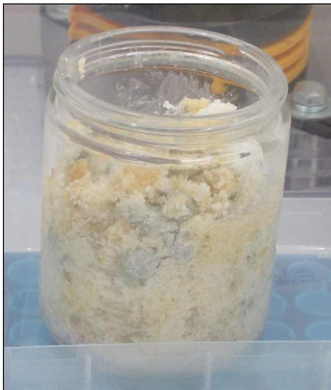
Figure 35. Solid reaction product formed from reaction of 100 mL VX with \text{Li}_3\text{N} + \text{H}_2\text{O} .
