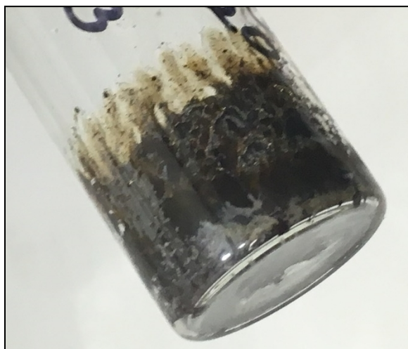
Figure 46. Reaction mixture of 10 mL GD + \text{Li}_3\text{N} + \text{H}_2\text{O} , using 10 mL GD, 9% \text{Li}_3\text{N} and 4% \text{H}_2\text{O} after 1 day of reaction time (sample NB0018P89B). The residual GD was below detection limits (<1%).
