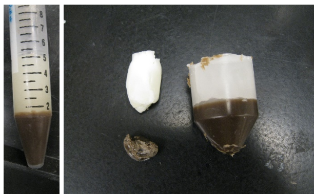
Figure 58. Centrifuged dust-encapsulated pellet after repeat melt/cool cycles. Headspace paraffin had discolored. The color change was pronounced compared to a sample prepared with a single melt process and allowed to settle/cool under ambient conditions.
