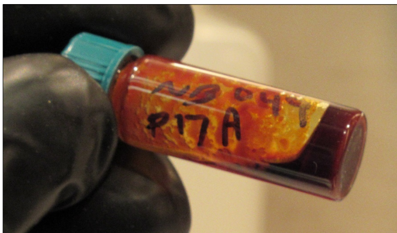
Figure 43. Reaction of HD with [(\text{CH}_3)_2\text{N}]_4\text{Ti} , sample NB0049P17A after two weeks of reaction time.
