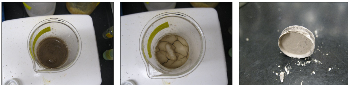
Figure 59. Progression of paraffin/dust/iso-octane slurry (left), dried powder (center) and pressed pellet (right).
