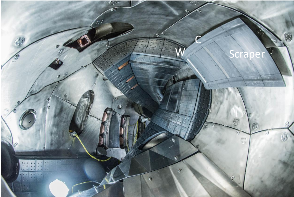
Fig. 7: View of a scraper element inside W7-X. The scraper has a W and a Mo/C marker layer close to the Langmuir probe arrays.
