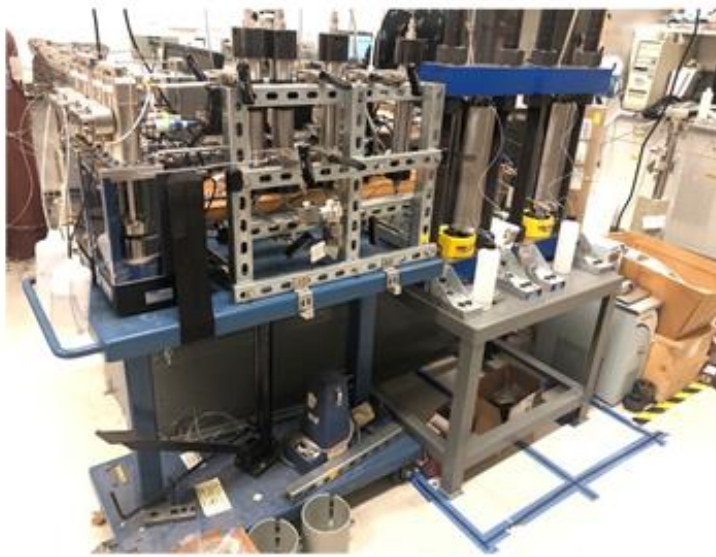
Dual-sample triaxial rock testing system
