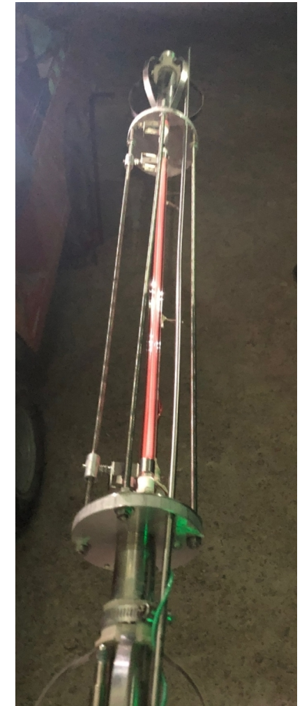
Infrared heater in BATS HP borehole
