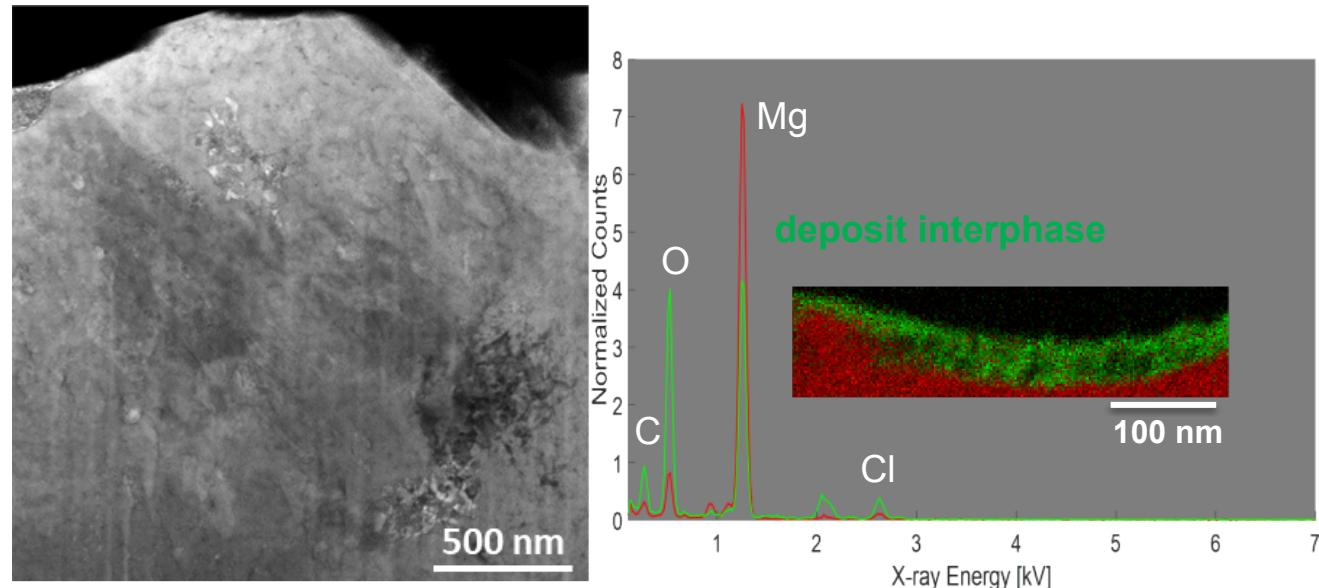
Epitaxial Mg deposition – same orientation within a grain from substrate to electrolyte interface
