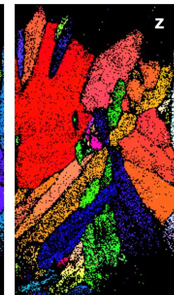
Trace  $\text{H}_2\text{O}$  directs greater degree of isotropic grain growth – water will be tied up in coordination with  $\text{Mg}^{2+}$  and this is the complex that is altering surface energetics.
