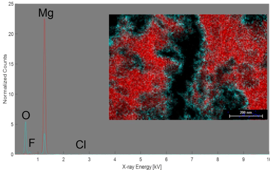
Dissolution pore walls are oxide capped
