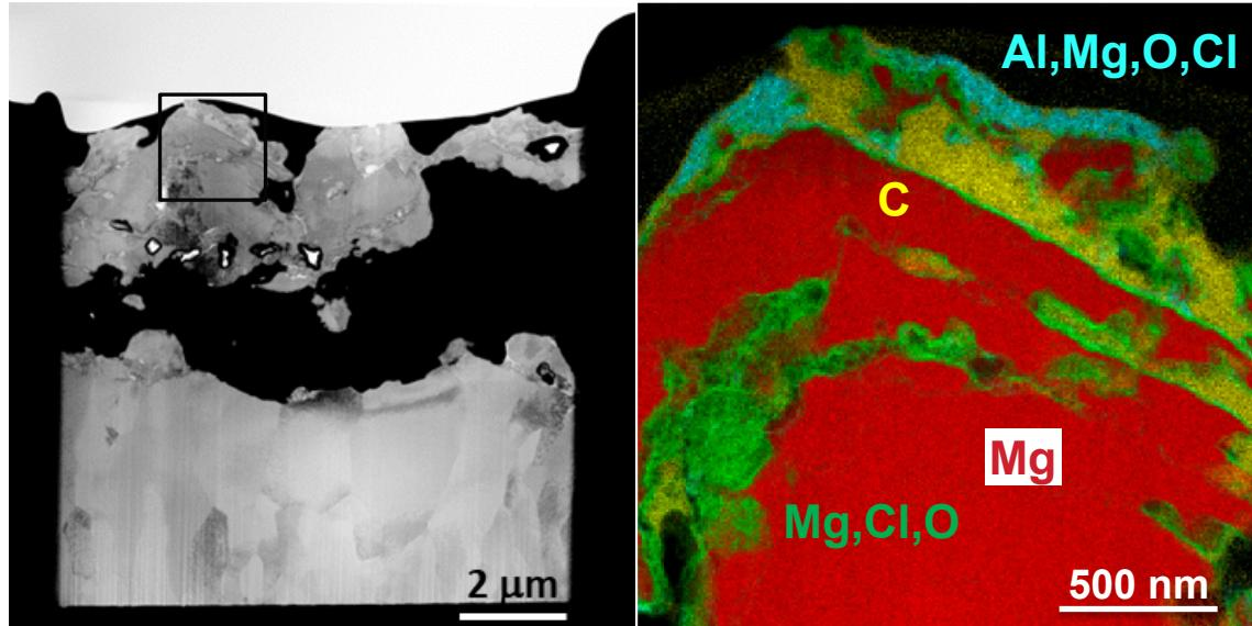
Accumulation of Al, O, Cl in a highly heterogeneous interphase
