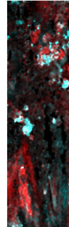
Capping oxide is crystalline, heterogeneous
