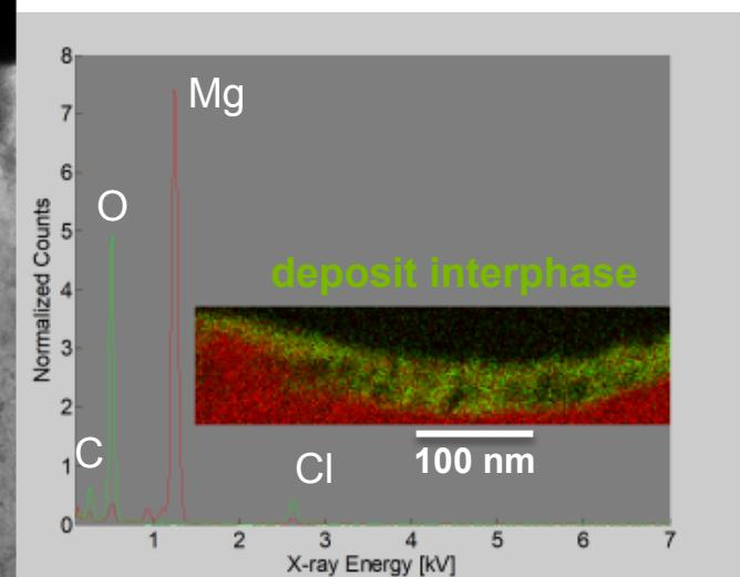
Epitaxial Mg deposition – no new interface, same orientation within a grain from substrate to electrolyte interface
