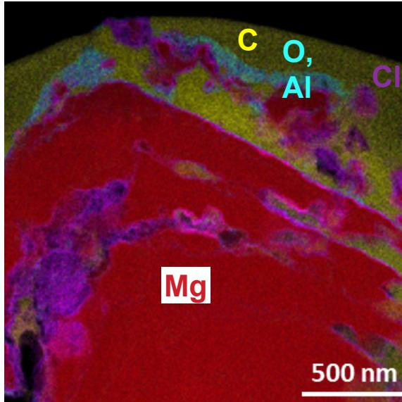
Accumulation of Al, O, Cl in a highly heterogeneous interphase
