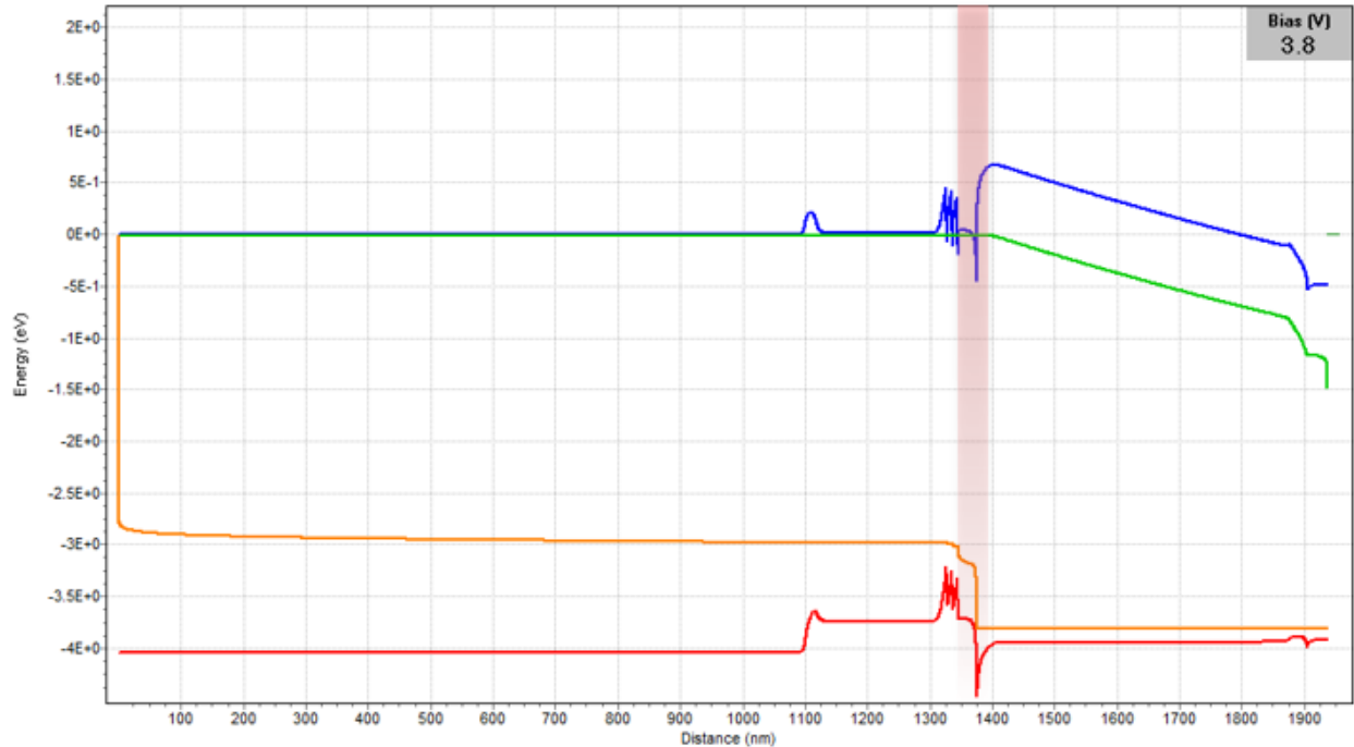
Figure 2-2. Band diagram of a LOC laser design with polarization doping grade in the p-cladding. Shaded region indicates a non-ideal transition from p-cladding to MQW.
