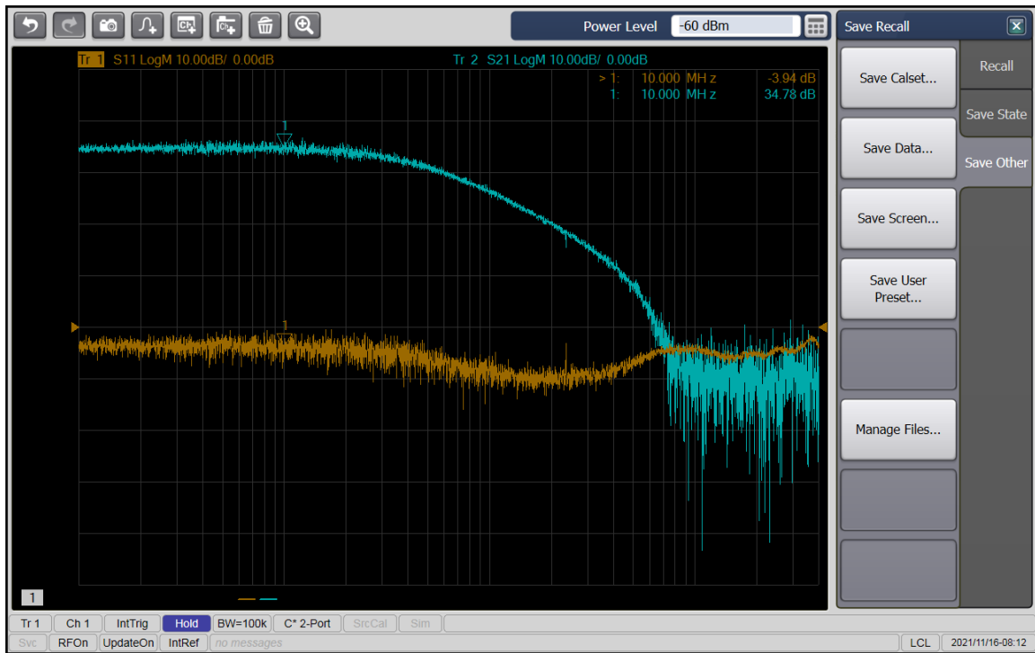
Figure 8. Measured 50 Ohm s-parameters of the modified SL55210TQFN-EVAL1Z.
