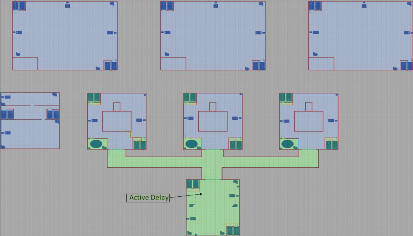
Figure 13 Active delay in the below-grade canister storage area
