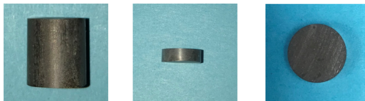
Figure I.1.1.4. Iron nitride based SMC containing 71.4 vol.% \text{Fe}_4\text{N} . In the images located in the center and right hand side, the sample has been cut using a diamond saw prior to insertion in a magnetometer.
