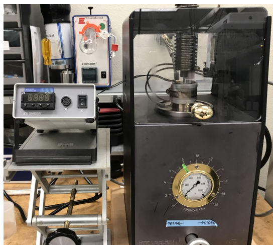
Figure I.1.1.1. Lab scale hot pressing setup used for SMC part fabrication.
