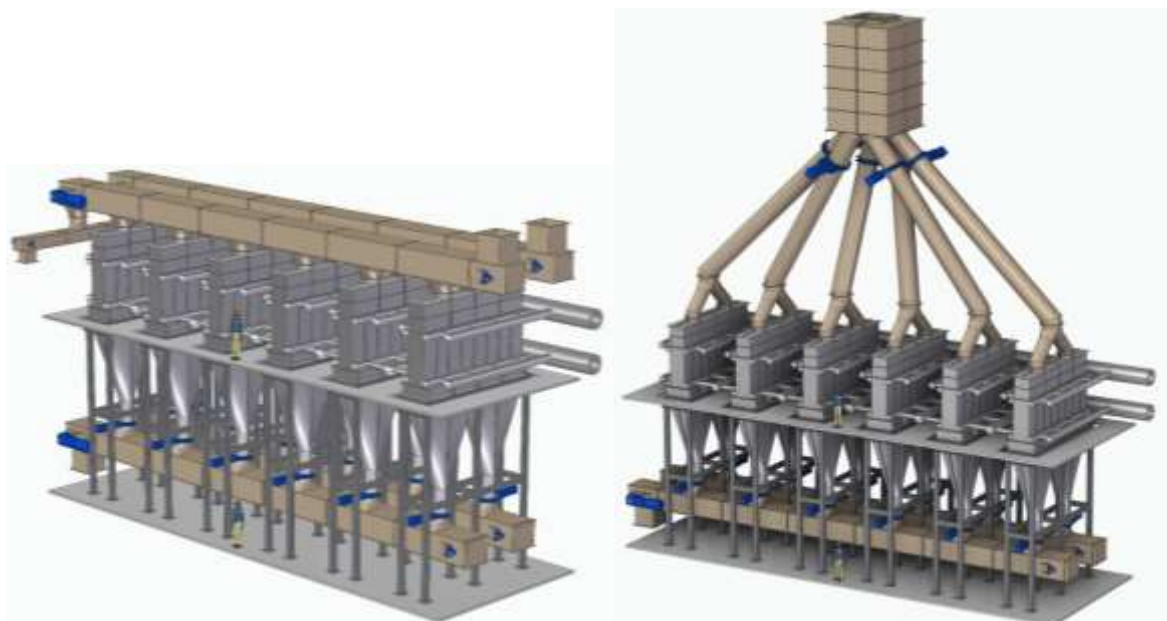
Figure 68. Two configurations for 200 MW t moving packed-bed particle-to-sCO 2 heat exchanger concept (6 x 33 MW t exchangers). Left: Drag-conveyor for ground-based system. Right: Gravity-driven feeder concept for tower-integrated or single-lift design. (Solex, VPE, and Sandia)
