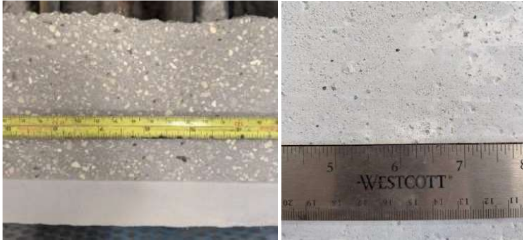
Figure 45. Left: Tuffcrete shows good adherence to Skamolex during shotcrete testing. Right: When Tuffcrete is pried off of Skamolex to simulate thermal expansion mismatch, there is minor damage (pitting), and no observable water damage.
