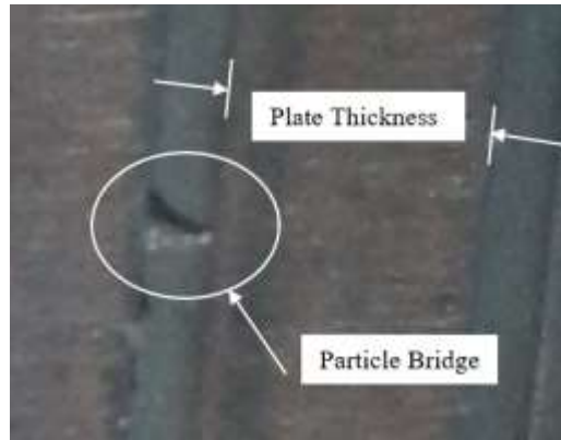
Figure 62. Particle bridging for 1/16" gap spacing
