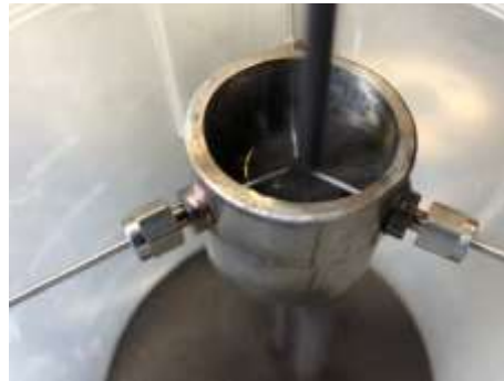
Figure 32. Nutted TC fixtures in radial array in early test demonstration
