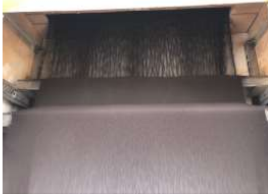
Figure 15. Particle flow over two troughs in receiver showing improvement in particle flow and opacity relative to free-fall particle flow and opacity above the troughs.
