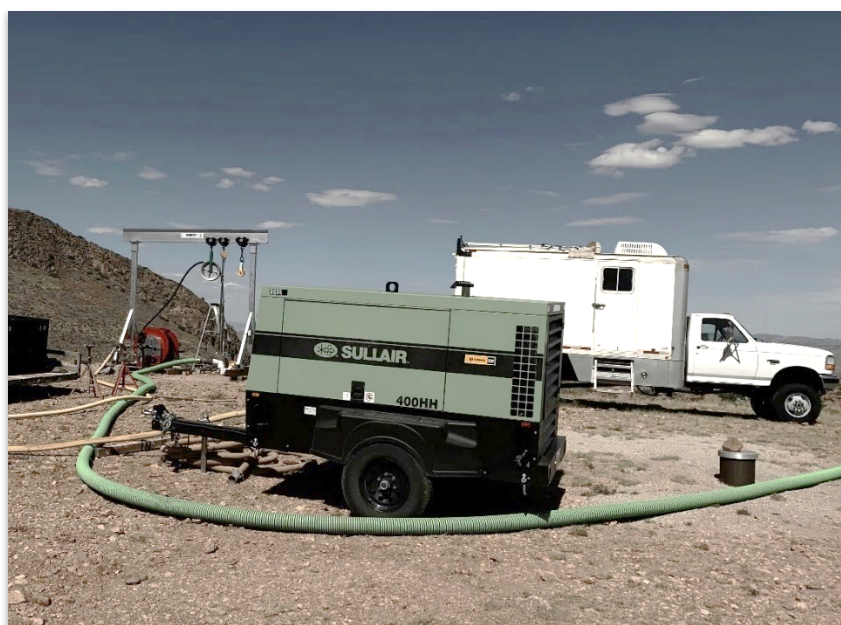
Figure 9-5. Air compressor used to drive hammer and motor (200 psi [ \sim 1,380 kPa], 400 scfm [ \sim 11.3 m 3 /min])
