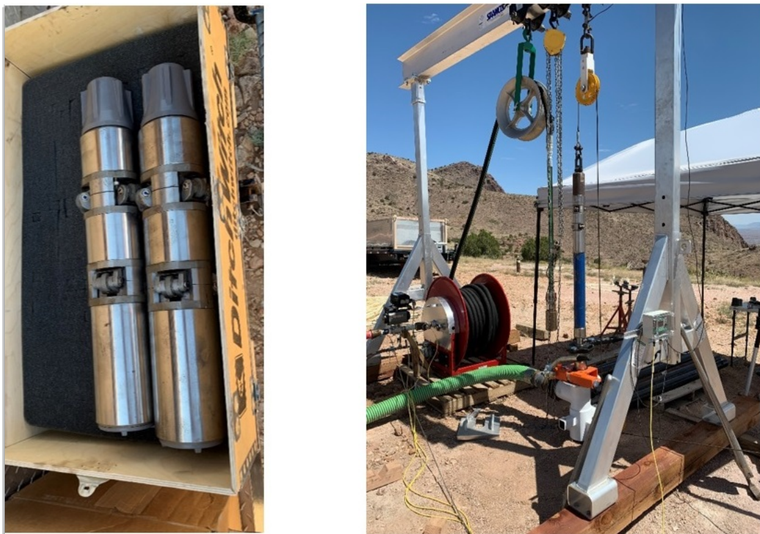
Figure 9-8. WOB modules (MADS) as built and assembled with two sets of reaction modules
