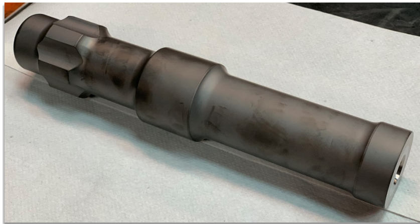
Figure 6-9. QLX 35 piston coated with DLC for solid lubrication
