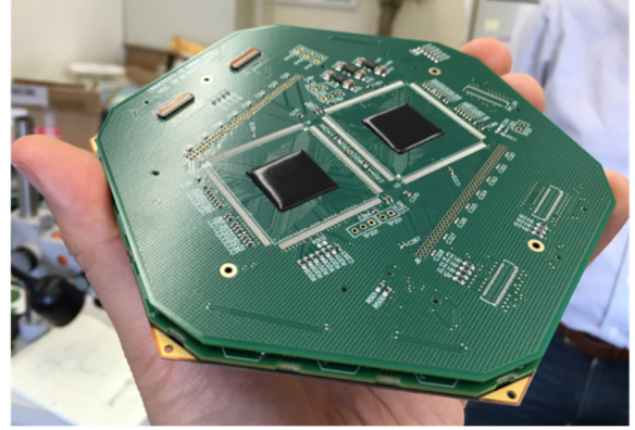
Figure 4. Photo of the complete HGCal module, with the readout board with two SKIROC2 bare die chips wire-bonded (under protective black potting material).
