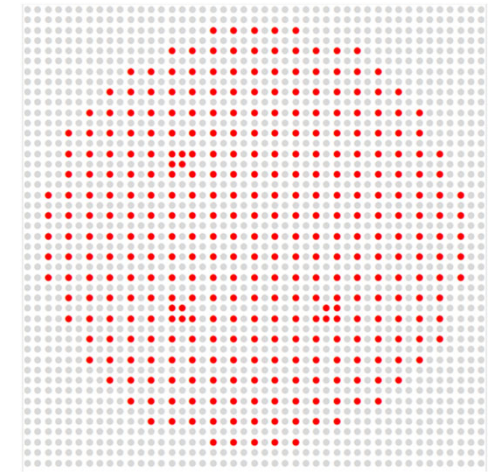
LCT102 Case 16 1.71 cm pitch 346 fuel rods Overmoderated
