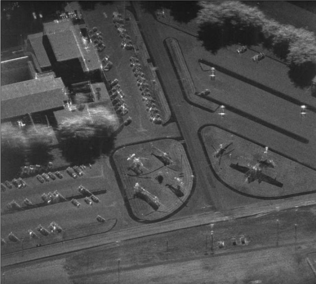
Figure 1. SAR image of a location at Kirtland Air Force Base, Albuquerque, N.M., exhibiting 4-inch (10 centimeter) resolution. Note that the aircraft are better defined by their shadows than by their direct echo return.
