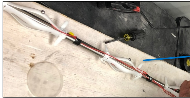
AE sensors on de-centralizers
