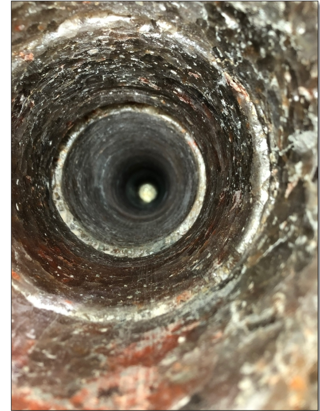
Discrete fractures in BATS near-drift EDZ
