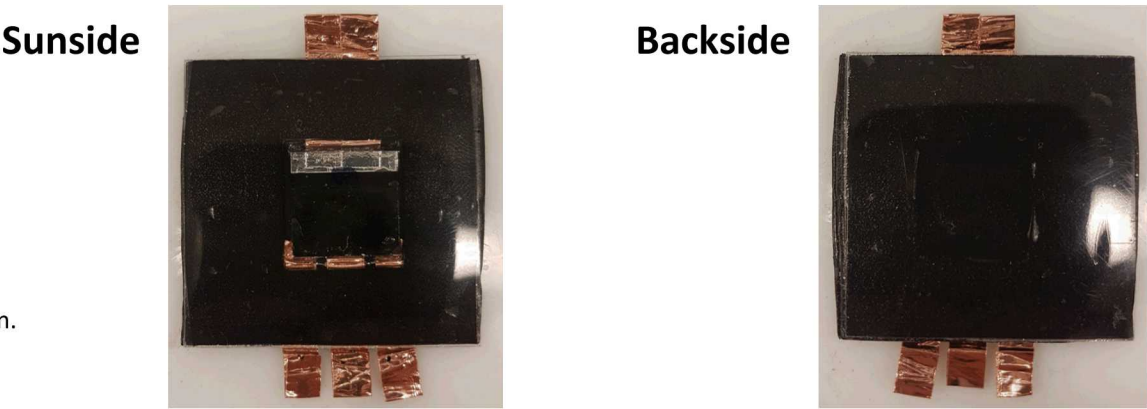
Figure 8. Encapsulation of PSC (a) In-house fabricated PSC, in collaboration with wide-bandgap PSC fabrication group at GT, (b) PSC efficiency measurements, where inset shows two connections to the Ag electrodes
