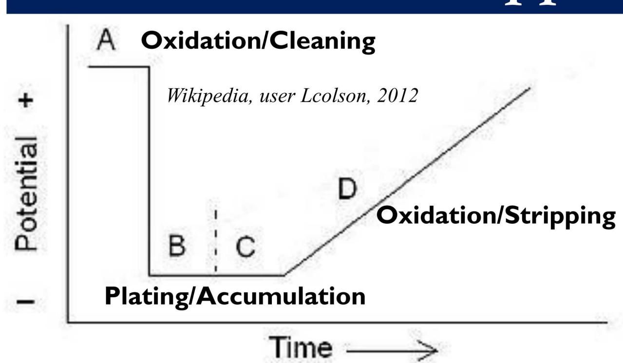
After an oxidative cleaning step, metal ions are plated onto the working electrode. Then, an oxidative potential is gradually applied, stripping the plated ions off the working electrode and generating a current which is measured.
