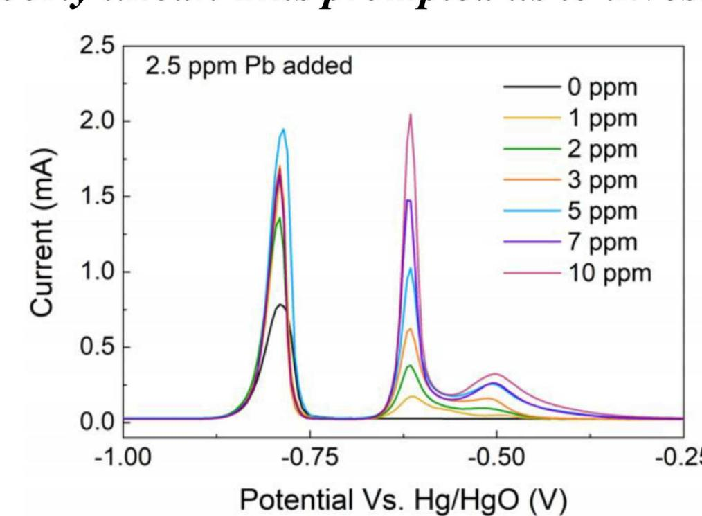
*A Pb mediator improves the linearity and repeatability of the calibration curve. Pb and Bi form an alloy on the electrode surface.*
