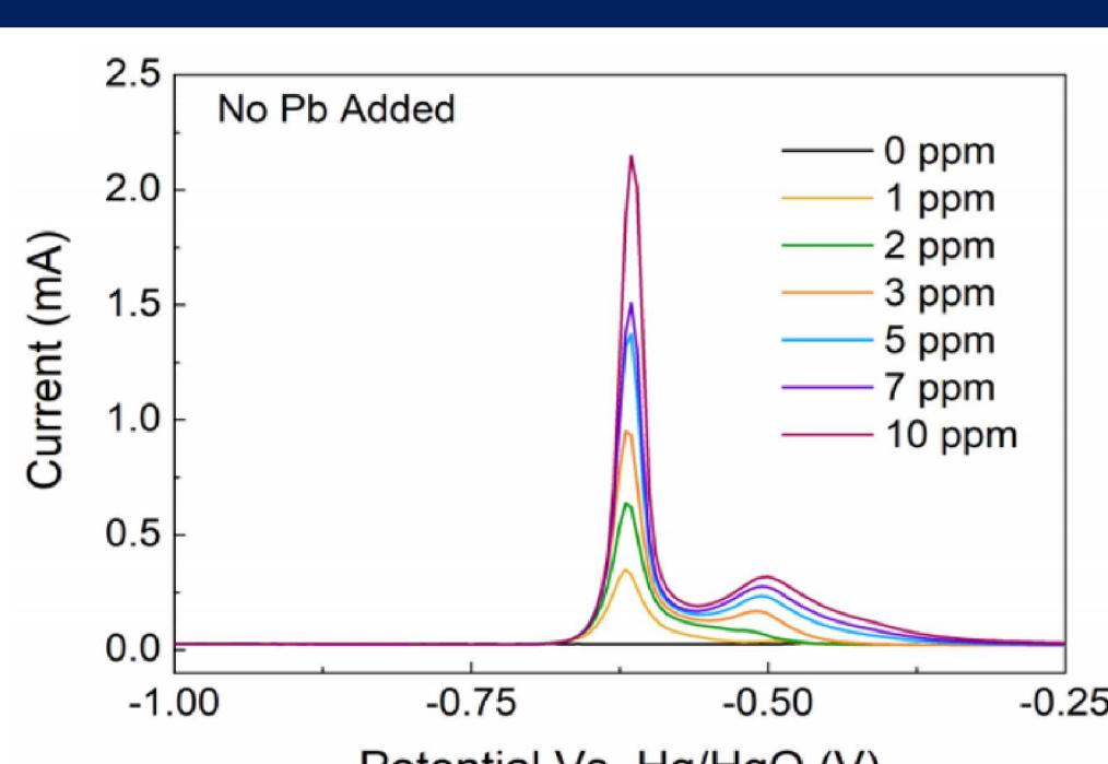
*Bi can be measured by itself in alkaline, however, the calibration curve we obtained was poorly linear. This prompted us to investigate the use of Pb as a stripping mediator:*
