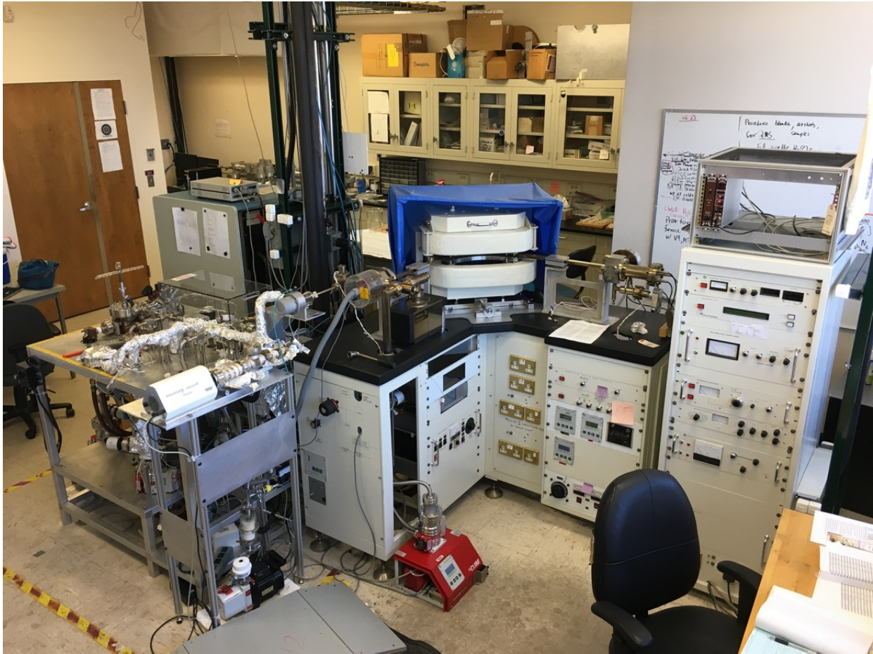
Figure 1: Photo of the Syracuse University Noble Gas Isotopic Research Laboratory showing the N purification line (with perplex cover; center left), noble gas extraction lines (covered in Al foil), Prisma quadrupole (white; left middle foreground) and Micromass 5400 noble gas mass spectrometer (right portion of photo). DOE Award # DE-SC0016246 provided funding for the fabrication and installation of the N purification line and modifications to the existing extraction line and mass spectrometers.
