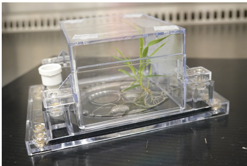
Fabricated ecosystems (EcoFAB) showing Brachypodium distachyon growing in hydroponic solution. Image credit: Kateryna Zhalnina. Image credit: Thor Swift/Berkeley Lab.
