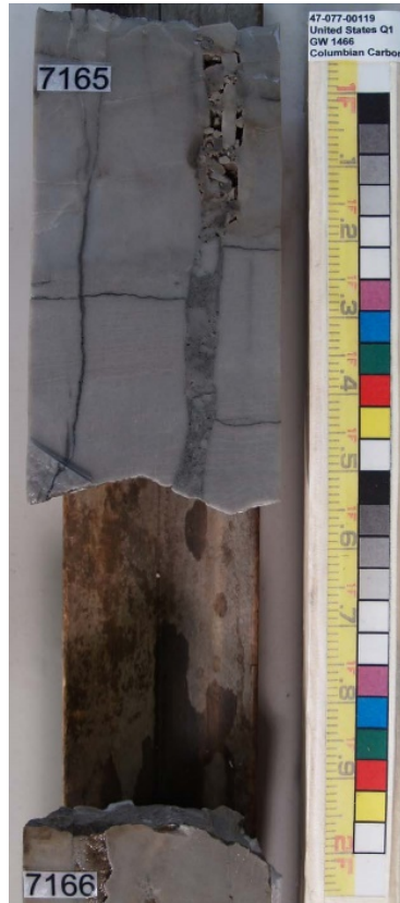
Figure 33: Whole cored interval taken from the bottom of the Tuscarora well test in the USA #Q-1-119. Core shows abundant fractures with visible porosity, likely extending up into the production-test interval.
