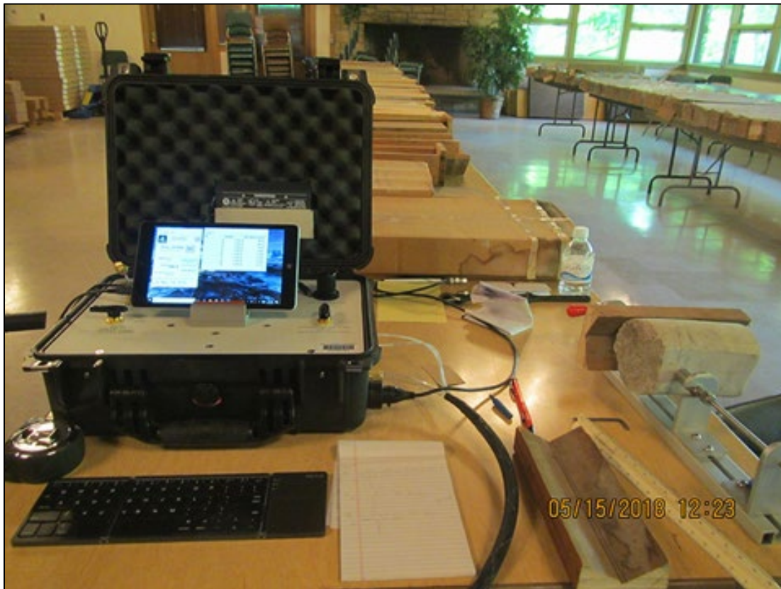
Figure 2: Core Labs PPP-250 Minipermeameter in operation. The instrument's probe is held tightly against the face of a core sample (on the right) while air is injected into the rock at approximately 26 psig. The instrument itself (on the left) measures the rate of gas uptake by the sample and computes the sample's permeability which is stored digitally on a small tablet computer (also on the left). The quantity being measured is k_{h\text{Air}} (horizontal permeability to air) in millidarcies (mD).
