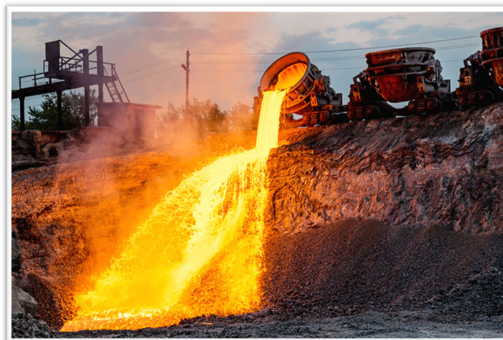
Figure 6-1. Iron slag being poured from slag pot.
