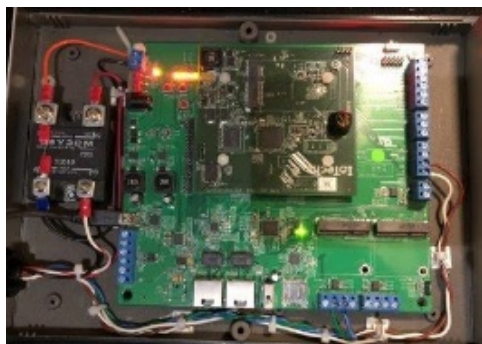
Figure 7: EV Communications Controller (EVCC) Chrysler Pacifica Van PHEV
