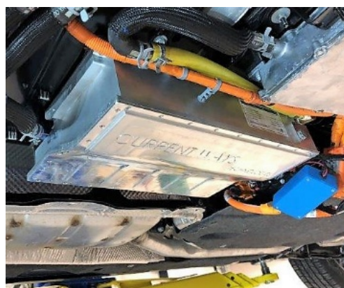
Figure 5: Bi-directional Charging Inverter Installed into Chrysler Pacifica Van PHEVs
