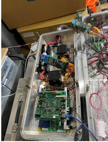
Figure 27 SPIN CCS Control Board Under Testing with Stellantis City EV EU Edition
