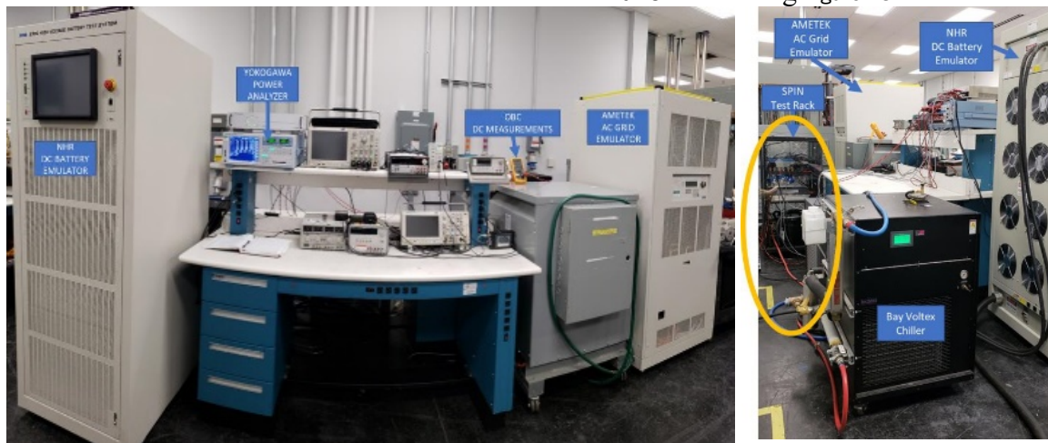
Figure 13: NTRC Lab Equipment Set Up with SPIN Rack System
