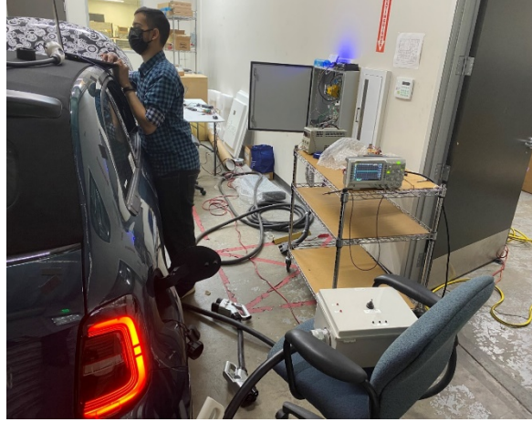
Figure 27 SPIN CCS Control Board Under Testing with Stellantis City EV EU Edition
