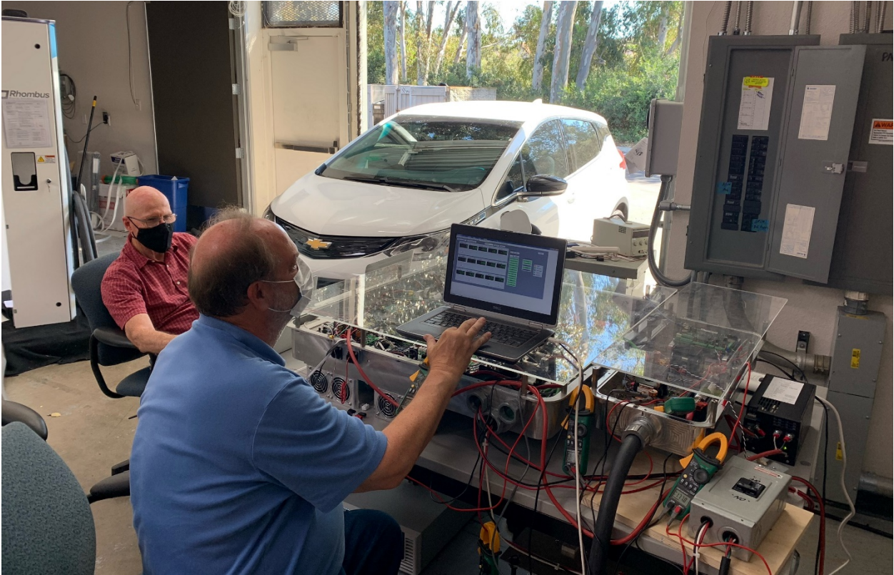
Figure 28 SPIN Setup for Integration with MY2020 Chevrolet Bolt EV
