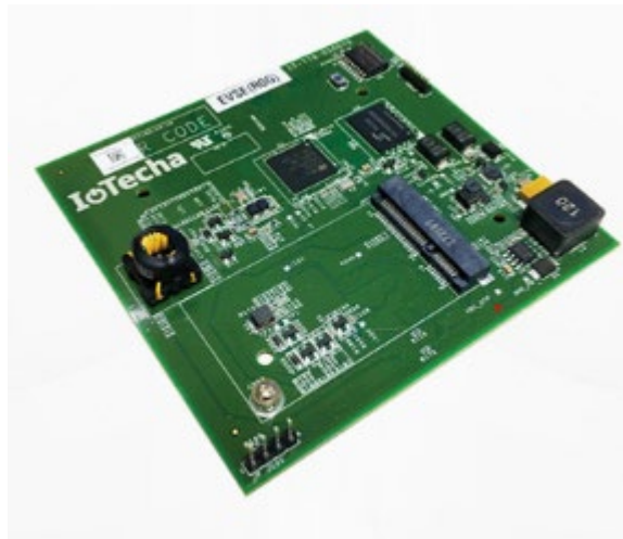
Figure 16 IoTecha EVCC and SECC Card Facilitates SPIN to PHEV DC Charging Communications (Source: IoTecha, Inc)
