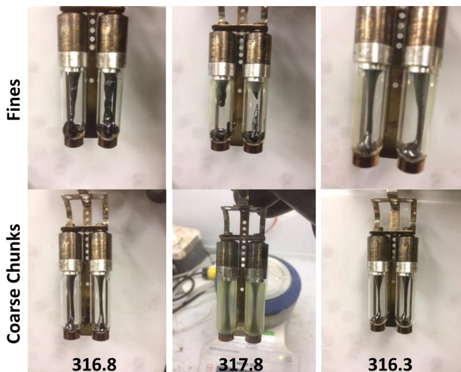
Figure 272: Photograph of scaled up Koppers PPM SP samples after analysis. SP samples of the fines are shown at the top and SP samples from the bulk chunks are shown at the bottom. Fines from the two samples on the left were heterogeneous and significantly different from the bulk (coarse chunks). The SP in °C is listed at the bottom of the bottom row of SP samples.
