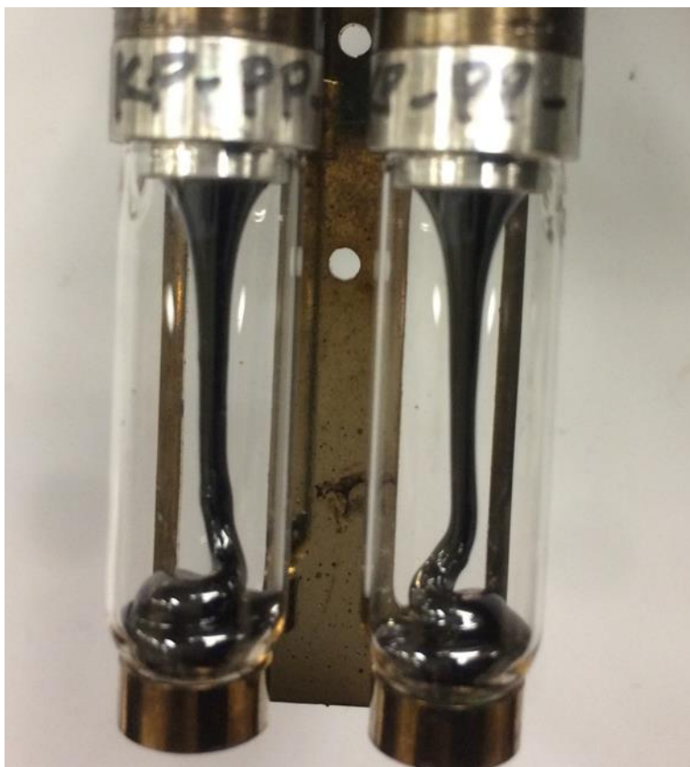
Figure 264: Photograph of the KPPM SP298 after SP determination.
