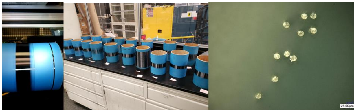
Figure 255: Left photo shows multifilament spinning of KP-PP-19. Middle photo shows several spools of as spun fibers produced under different conditions to reduce the CF diameter. Right photo shows as spun fibers with a diameter less than 25 \mu\text{m} .
