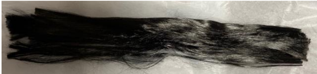
Figure 188: ORNL pitch fiber sent to UW, (CTP6M SP315+).
