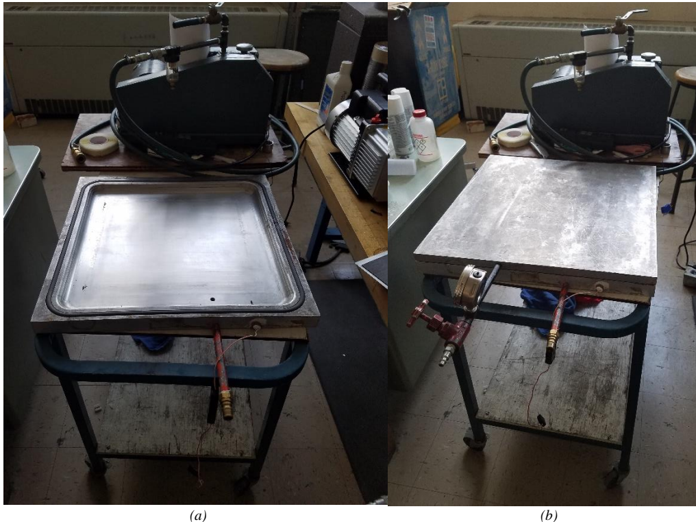
Figure 147: Pressure clave interior (a), and with top plate (b).
