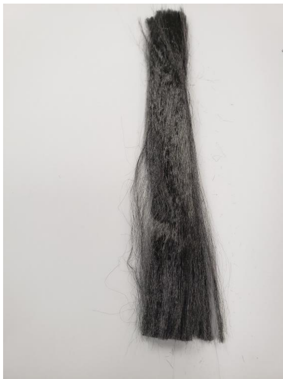
Figure 260: Approximately 12 g bundle of petroleum mesophase pitch carbon fiber sent to UW for composite testing.
