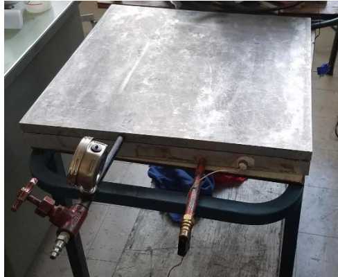
Figure 150: A photograph of the press-clave used for this work.
