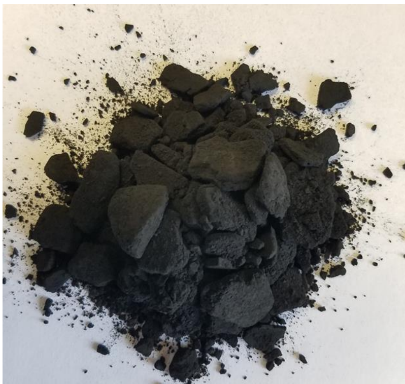
Figure 267: Dried primary-QI (2.3 %) from initial Koppers PP (500 g) that was insoluble in NMP and collected by filtration.
