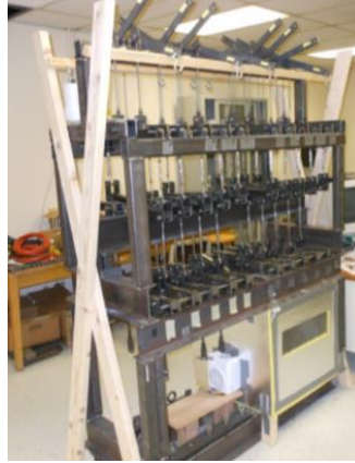
Figure 186: Image of creep frame system
