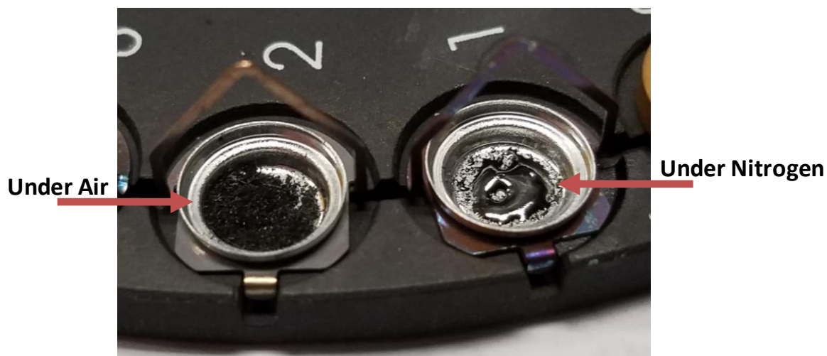
Figure 35: Photograph showing isothermal TGA (300-350 °C) of green fibers from CTP6M SP320 performed under air (left) which retains the structure of the crushed fibers and the experiment performed under nitrogen (right) resulting in complete melting of the fibers.
