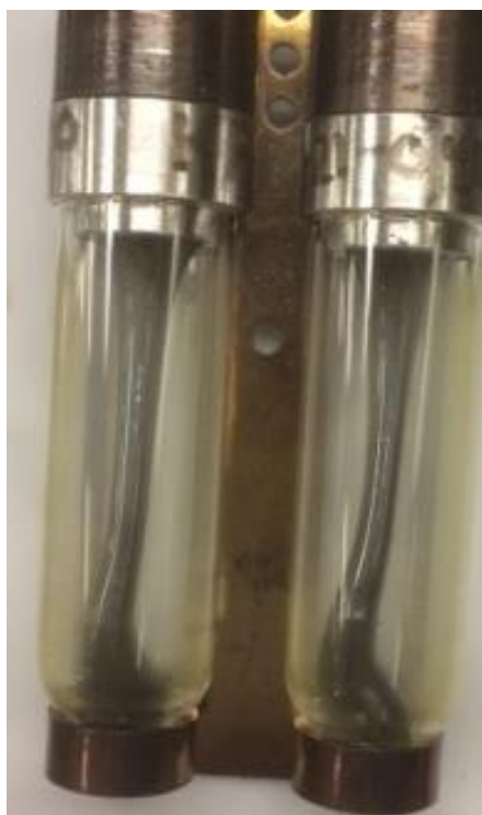
Figure 270: Photograph of the SP sample for KP-MP-21-0480. Yellow haze on the glass of the SP test vials indicates the presence of volatiles.
