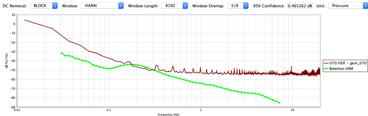
Figure 49 Self-Noise Power Spectra, Gem Package #070
