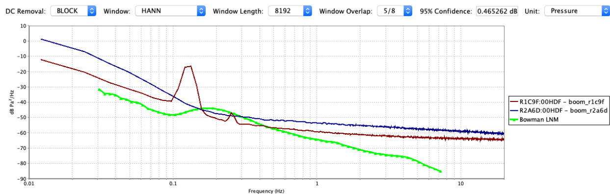
Figure 51 Self-Noise Power Spectra, Raspberry Boom Packages
