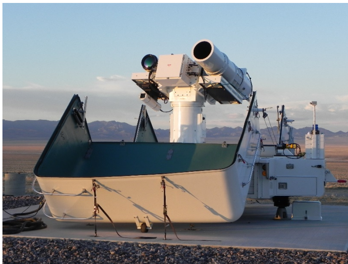
Figure 1-1. Gimballing Tracking Mount (GTM)
