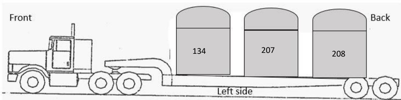
Notes: TRUPACT #208 is empty. Dose rates recorded on the front, back, left, right, top, and bottom are the highest detectable dose rates for that side/area. Dose rate survey performed in occupied areas of the cab.
