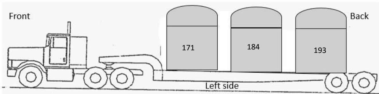
Notes: TRUPACT #193 is empty. Dose rates recorded on the front, back, left, right, top, and bottom are the highest detectable dose rates for that side/area. Dose rate survey performed in occupied areas of the cab.
