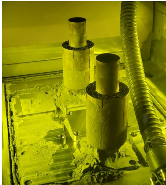
Figure 6. Parts during additive manufacturing process
