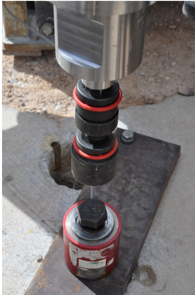
Figure 9. Load cell and bolt torque test fixture
