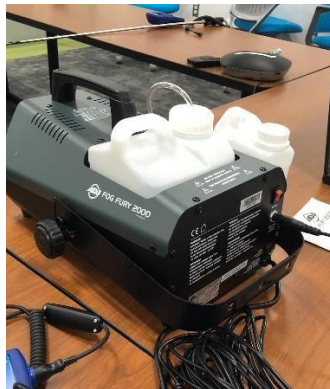
Figure 16. Fog machine used for smoke purge testing
