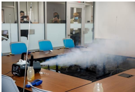
Figure 24. Purge test using emissions from fog machine
