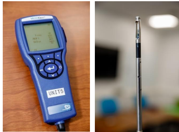
Figure 13. Meter and thermoanemometer tools used for testing
