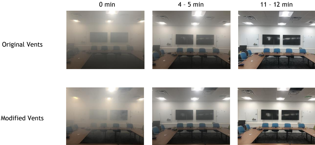
Figure 28. Sequence of images during fog-purge tests at ~600 cfm.
