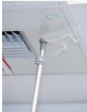
Figure 22. Tissue Test Tool used to understand airflow direction
