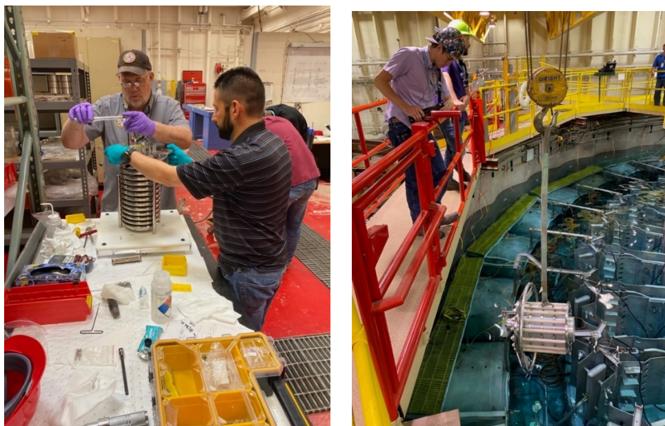
Figure 2. A new Saturn switch being assembled (left) and lowered into the Saturn water tank (right).
