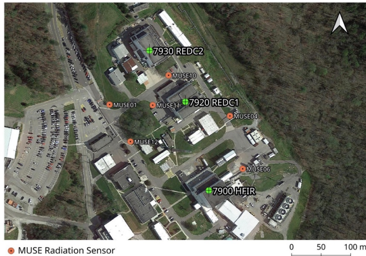
Figure 1. Map of radiation sensors distributed around HFIR and REDC to analyze transfers of material between facilities.
