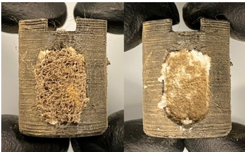
Figure 5. Photographs of Sample F-1, Site B, within the polymer sample head, before (left) and after (right) removal of the upper Scotch-brite® pad.
