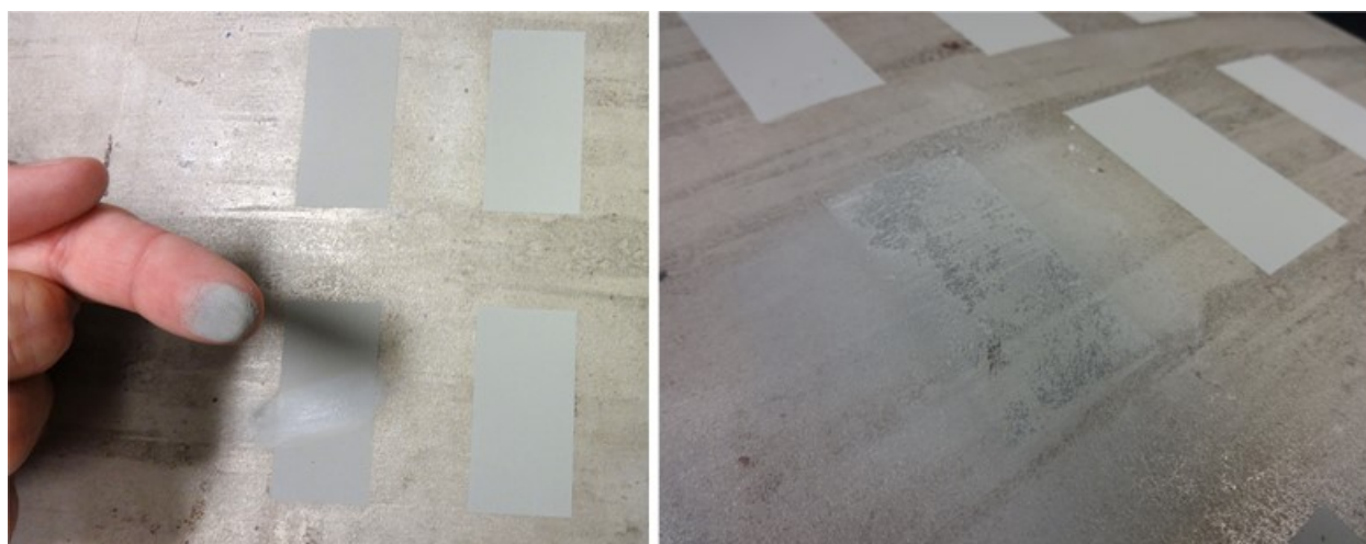
Figure 46. Degradation of the enamel markings after two weeks at 200 °C.
