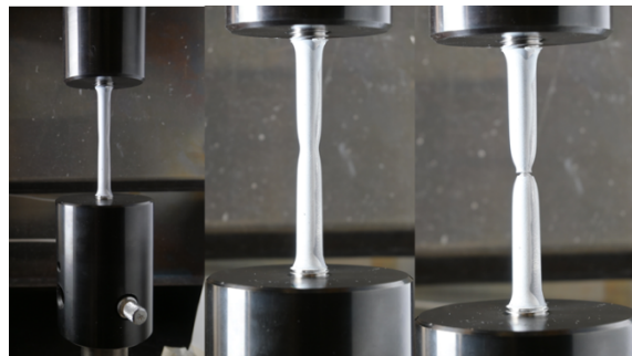
Figure 106. Example progression of tensile tests on round tensile specimens. The white coating is a random speckle pattern for Digital Image Correlation strain measurement.
