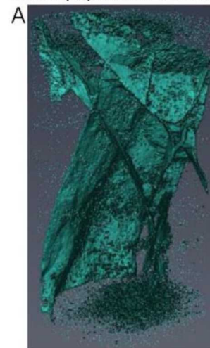
Segmented MicroCT images of failed samples
