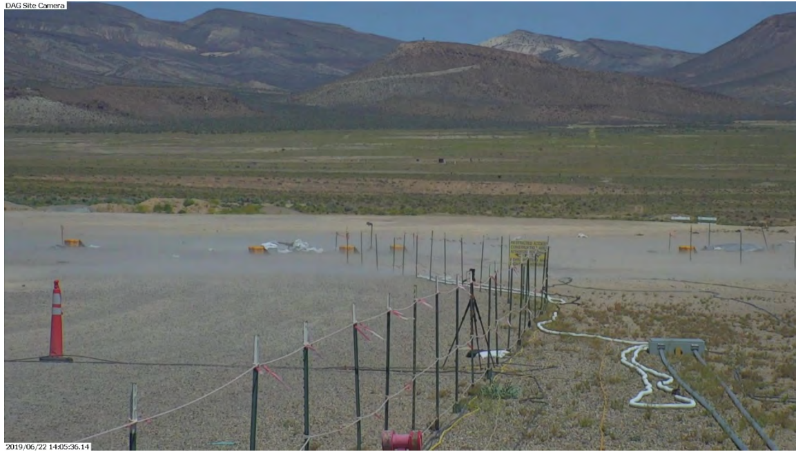
Figure 12. DAG-4 shot from the site camera; minor ground heave due to the blast launches dust from the ground.
