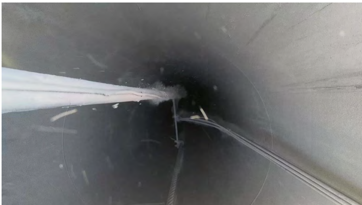
Figure 4. DAG-2 shot from GoPro 2, directed down the U2ez hole; dust is released from the cables due to the explosive blast.
