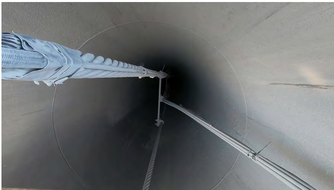
Figure 7. DAG-3 shot from GoPro 1; debris is knocked from the cables by the explosive blast.
