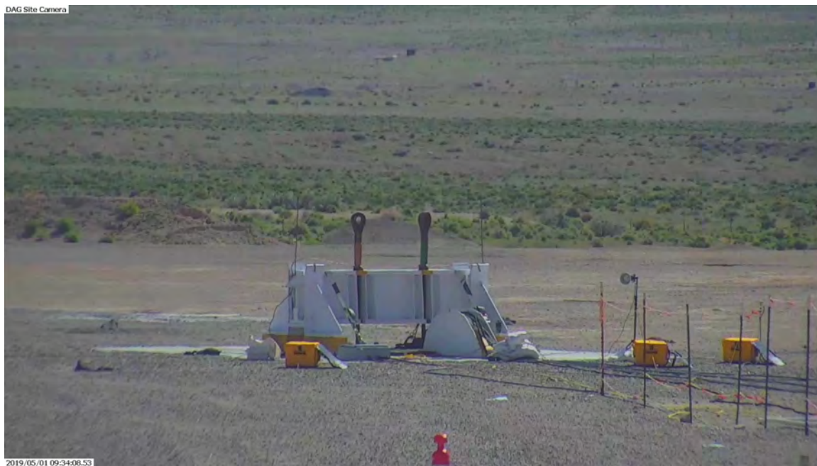
Figure 9. DAG-3 cable cutters from the site camera; camera shake indicates shot occurred.
