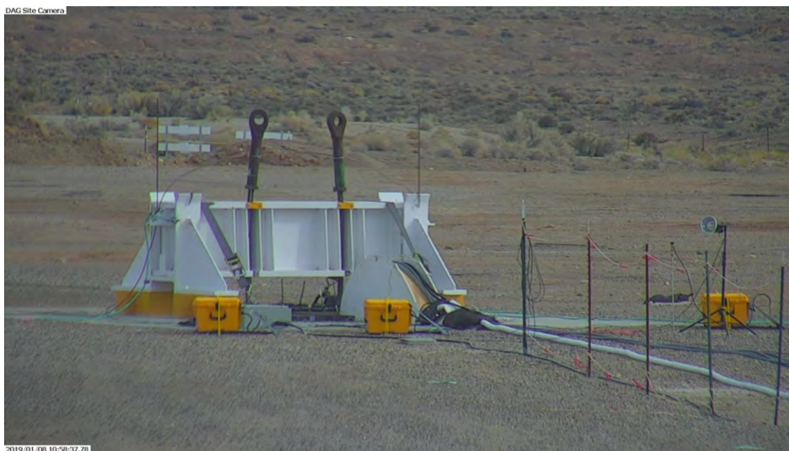
Figure 5. DAG-2 cable cutters from the site camera; cable “hop” can be seen as tension is released from the wires.
