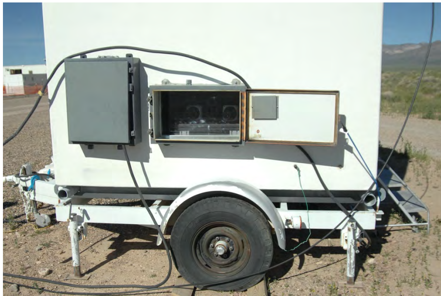
Figure 1: Trailer (Ice Box) to house high-speed cameras and other equipment.
