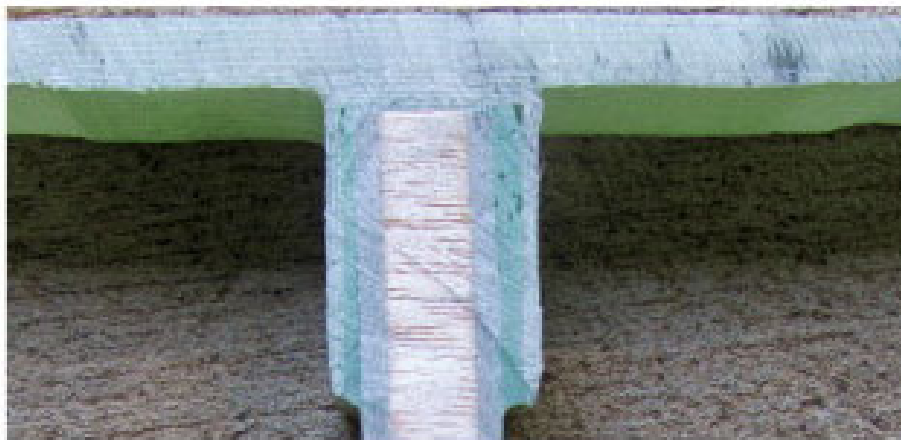
Figure 3-11. Cross-section of manufactured Pi joint.
