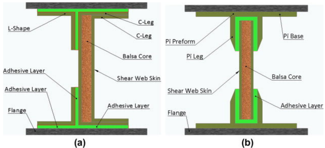
Figure 3-10. a) “C with L” joint and b) Pi joint [73].
