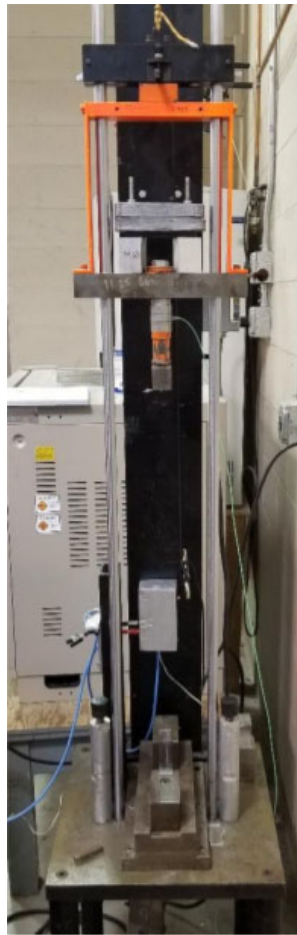
Figure 2-3. Impact tower setup [23].
