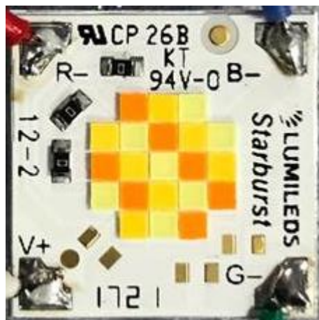
Figure 16: Tunable CCT demonstration module. The 1414 prototype LEDs are assembled at a pitch of 1.5 mm.
