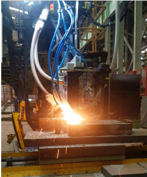
Automated cladding machine at Doosan
