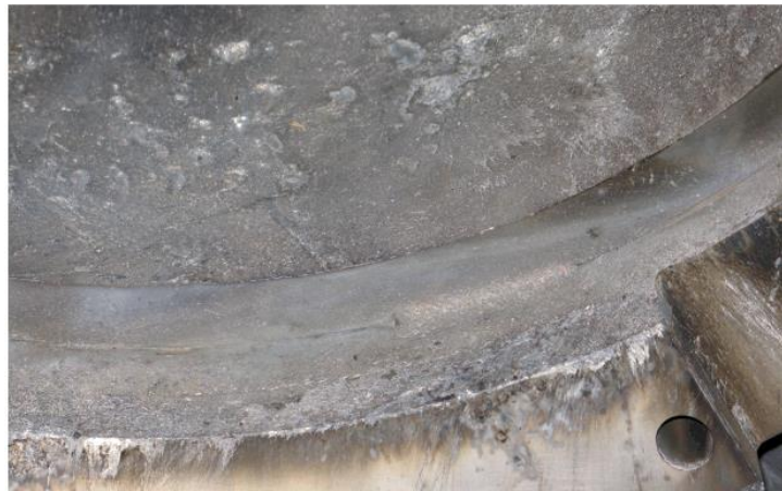
Figure 3-1. Top left: Image from an alignment camera during a Z shot. Top right: Image of the damage to the load hardware following a Z experiment. Bottom: Aftermath of two types of debris, including molten spray (left) and bullets (right).
