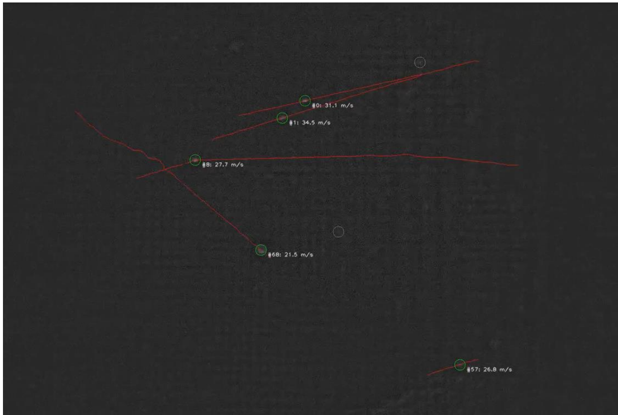
Figure 3-11. Tracking of debris particles early time (33 ms).
