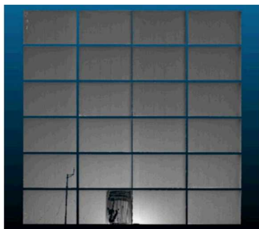
Figure 7. Heliostat scan with partially clean facet on bottom row.
