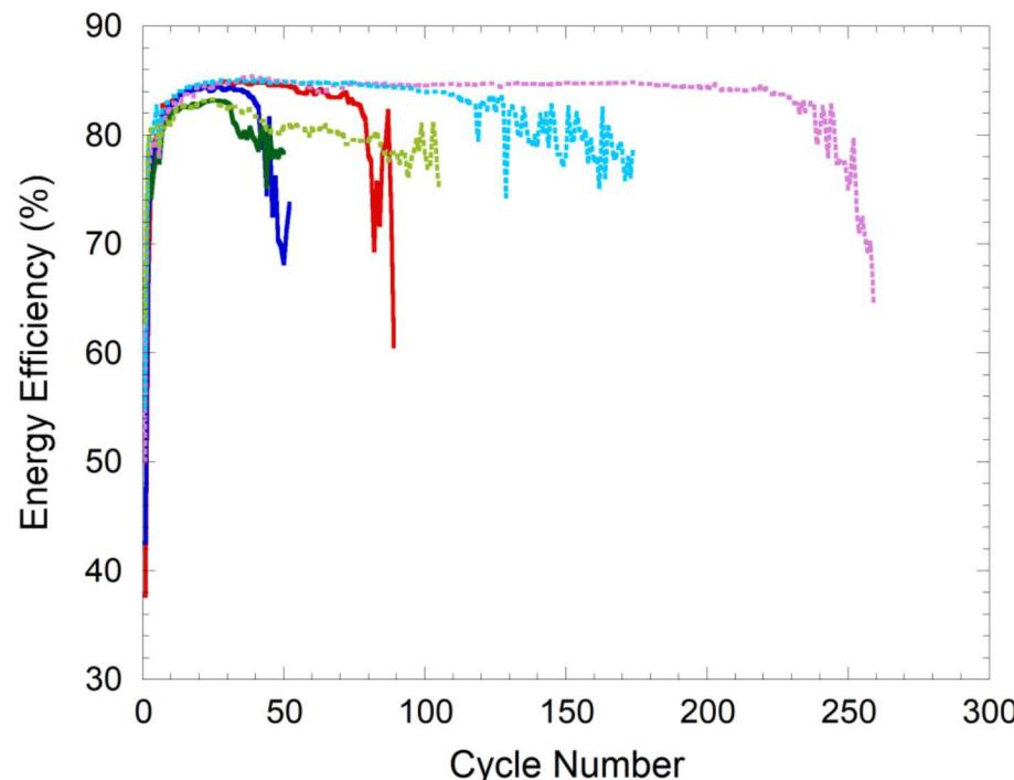
Cells with ZnO-saturated electrolyte last significantly longer with similar energy efficiency to cells with regular electrolyte cycled at same DOD, even *when including dissolved ZnO in capacity*
