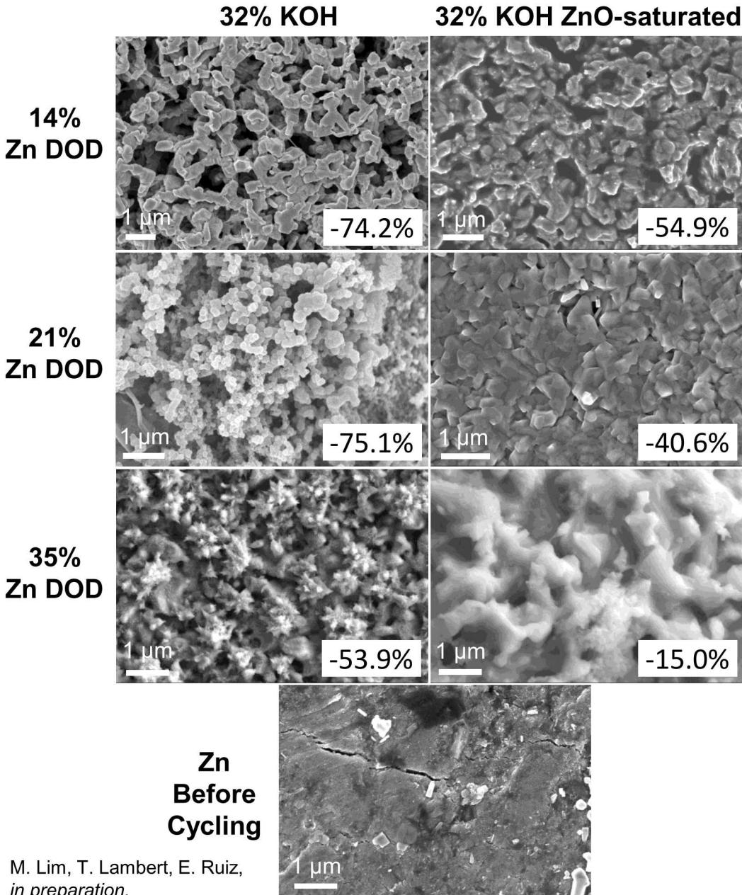
Cells disassembled in charged state following failure (80% of nominal cycled capacity).
