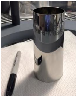
Figure 9: Picture of the first test optic for a future NIF Wolter microscope.
